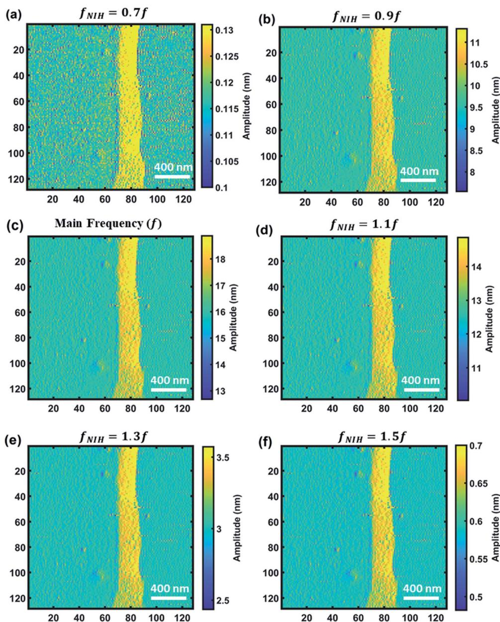
Fig. 8 Non-integer harmonic images of sample 1. (a) Amplitude image at  $0.7f$  (51 kHz), (b) amplitude image at  $0.9f$  (65.6 kHz), (c) amplitude image at the main frequency ( $f = 72.96$  kHz), (d) amplitude image at  $1.1f$  (80.2 kHz), (e) amplitude image at  $1.3f$  (94.8 kHz), and (f) amplitude image at  $1.5f$  (109.4 kHz).
