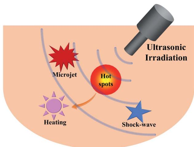
Fig. 3 Physical and/or mechanical effects from acoustic cavitation in a liquid.
