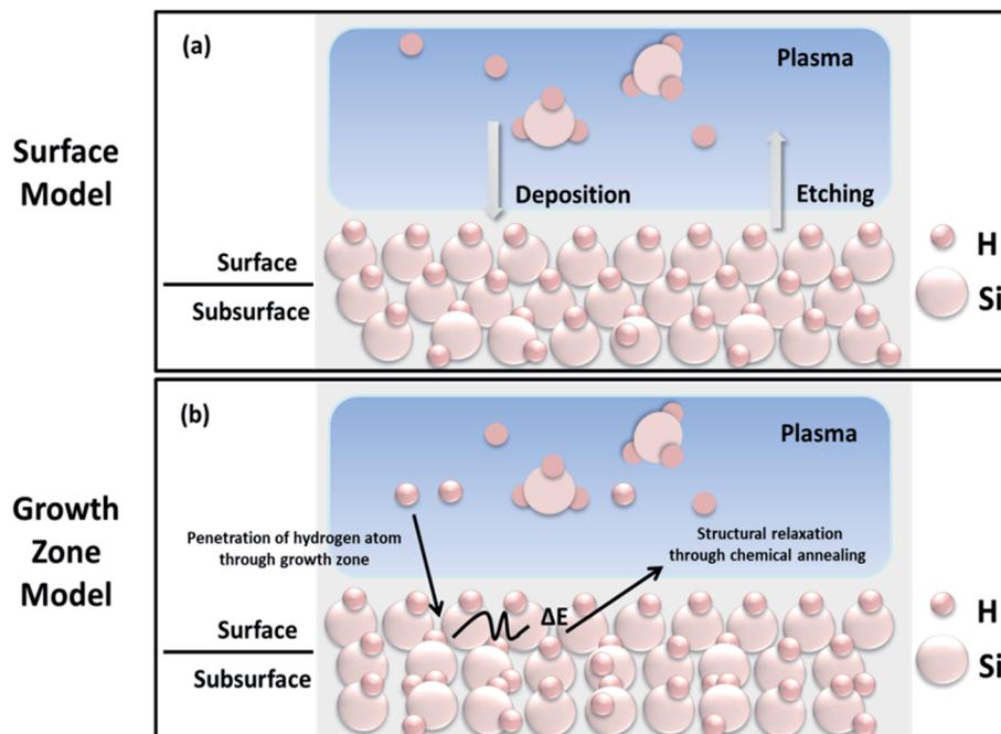
Fig. 4 Schematic representation of (a) the surface model and (b) growth zone models for the growth of nc-Si:H thin films.<sup>18,30</sup>
