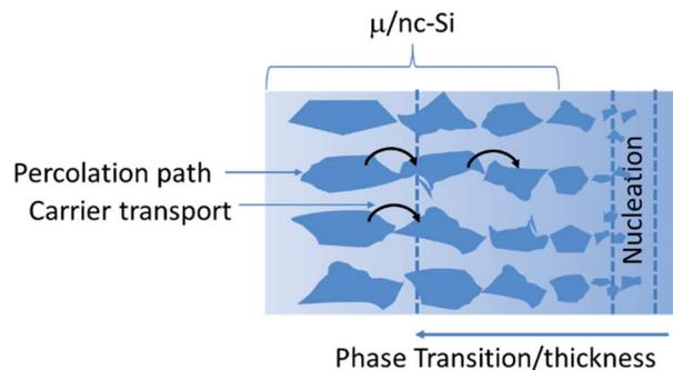
Fig. 6 Schematic representation of film thickness dependent carrier transport mechanism *via* silicon micro-/nano-crystallites embedded in an amorphous silicon matrix.<sup>23</sup>
