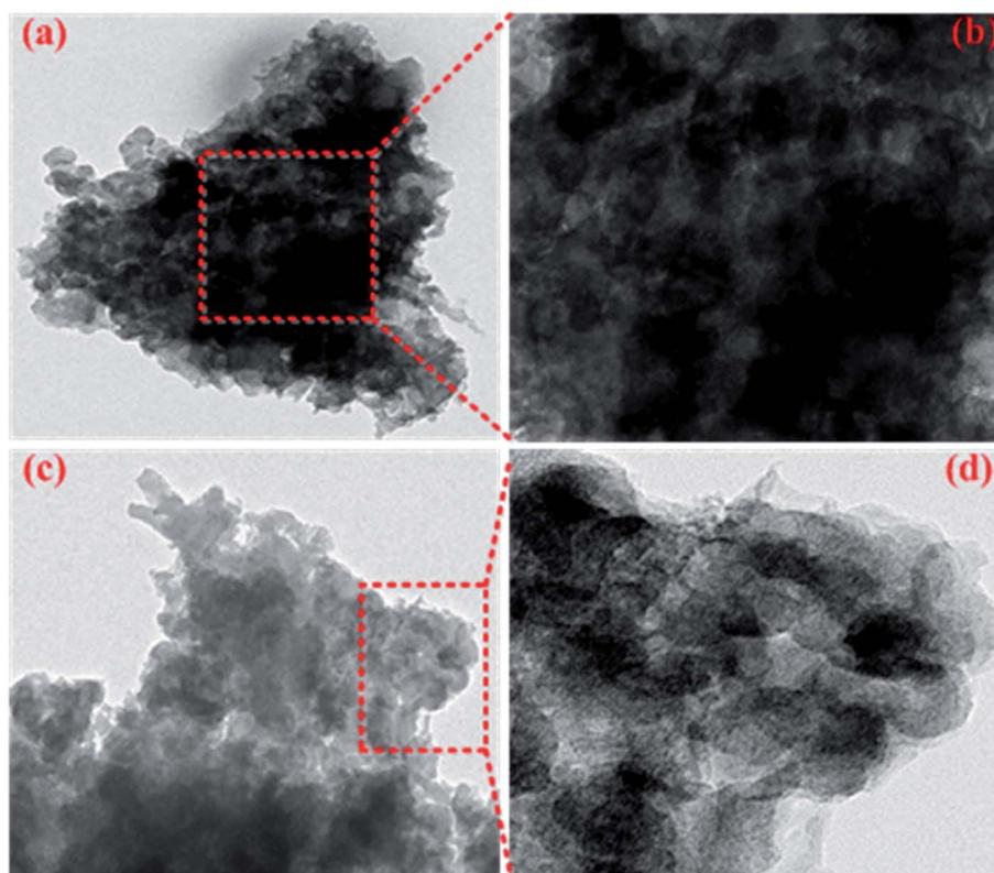
Fig. 15 TEM images of NTCDA electrodes (a and b) and TNTCDA-NiPc electrodes (c and d) after 400 cycles.
