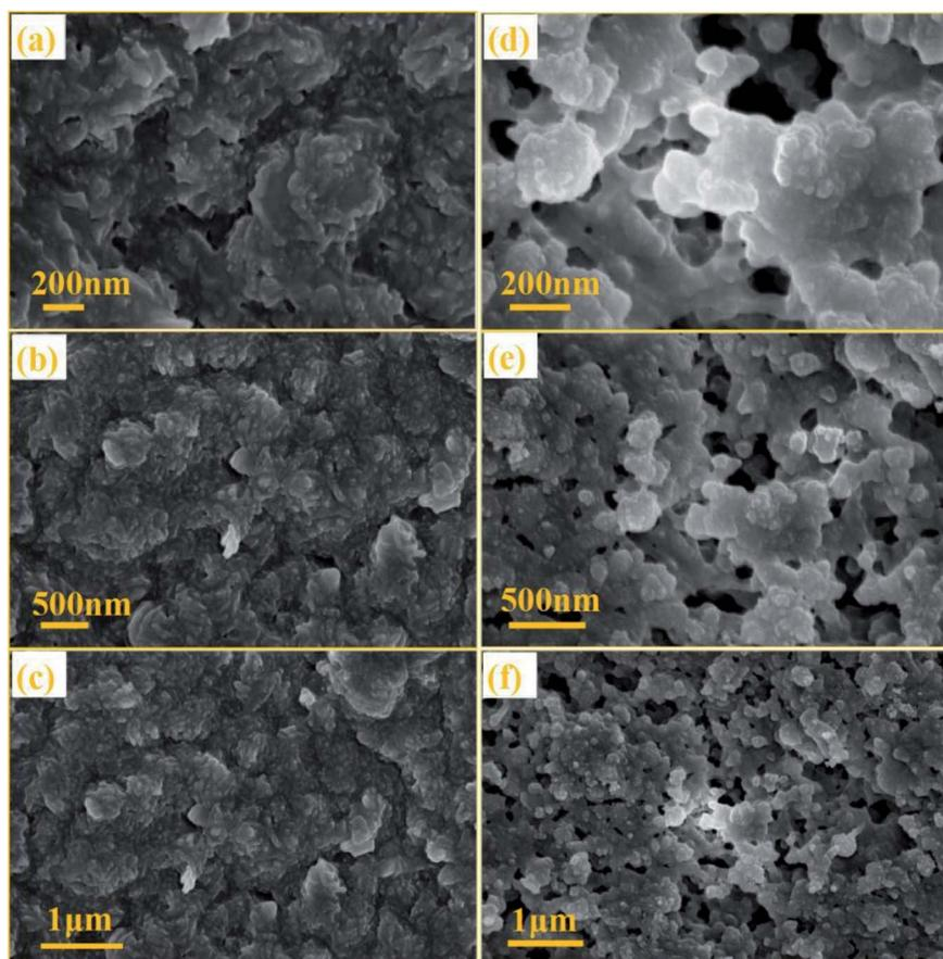
Fig. 14 SEM images of **NTCDA** electrodes (a–c) and **TNTCDA-NiPc** electrodes (d–f) after 400 cycles.
