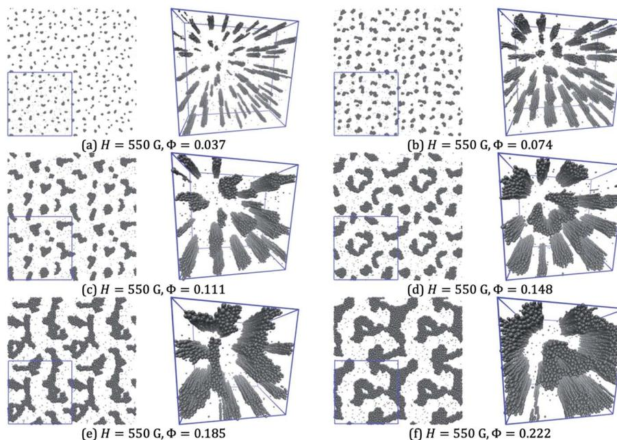
Fig. 16 Snapshots from simulations with  $H = 550$  G and (a)  $\Phi = 0.037$ , (b)  $\Phi = 0.074$ , (c)  $\Phi = 0.111$ , (d)  $\Phi = 0.148$ , (e)  $\Phi = 0.185$ , and (f)  $\Phi = 0.222$ . In each case, an orthographic view (with 4 periodic replicas) and a perspective view are shown.
