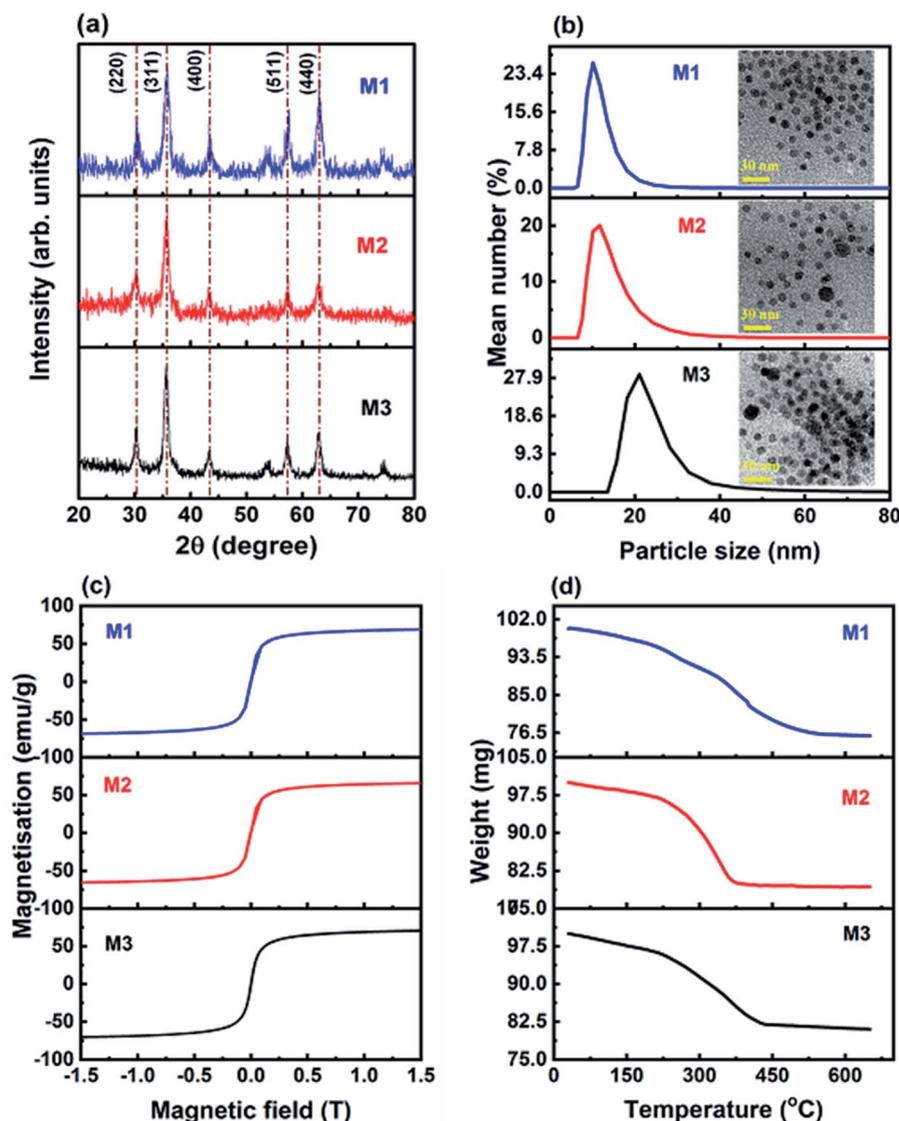
Fig. 1 (a) X-ray diffraction pattern of M1, M2 and M3. (b) Hydrodynamic size distribution of M1, M2 and M3 and (insets) their TEM images, (c) M–H curve of M1, M2 and M3, and (d) thermogravimetric weight loss curves of the dried surfactant coated magnetite nanoparticles of M1, M2 and M3.
