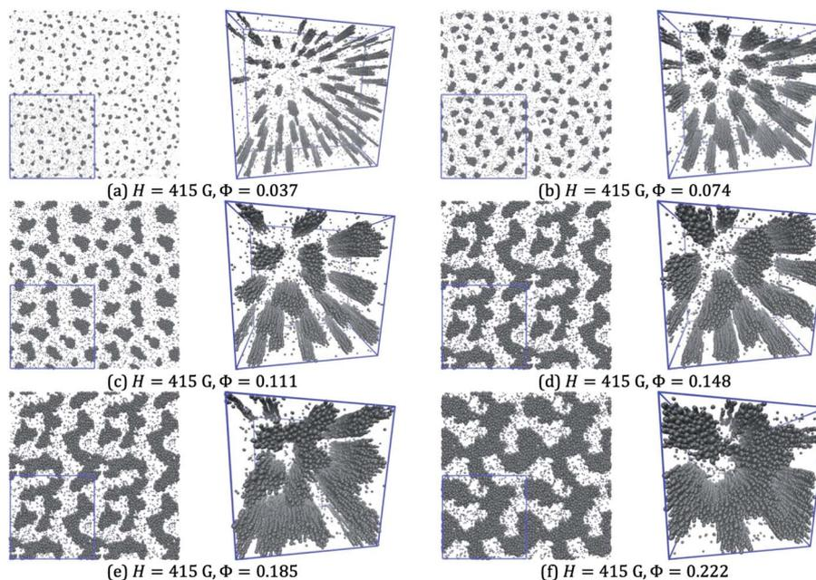
Fig. 15 Snapshots from simulations with  $H = 415$  G and (a)  $\Phi = 0.037$ , (b)  $\Phi = 0.074$ , (c)  $\Phi = 0.111$ , (d)  $\Phi = 0.148$ , (e)  $\Phi = 0.185$ , and (f)  $\Phi = 0.222$ . In each case, an orthographic view (with 4 periodic replicas) and a perspective view are shown.
