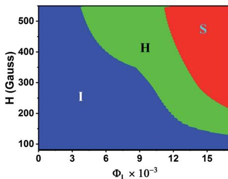
Fig. 9 Phase diagram of magnetic nanofluids with the large-particle volume fraction  $\Phi_L$  and magnetic field strength  $H$ , showing the structural boundaries between isotropic (I), hexagonal (H), and stripe (S) phases.
