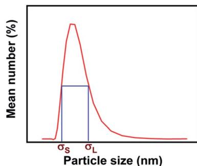
**Fig. 5** The particle-size distribution curve and the full width at half of the maximum intersect at two points, which define the hydrodynamic diameters of the small particles ( $\sigma_s$ ) and the large particles ( $\sigma_L$ ).
