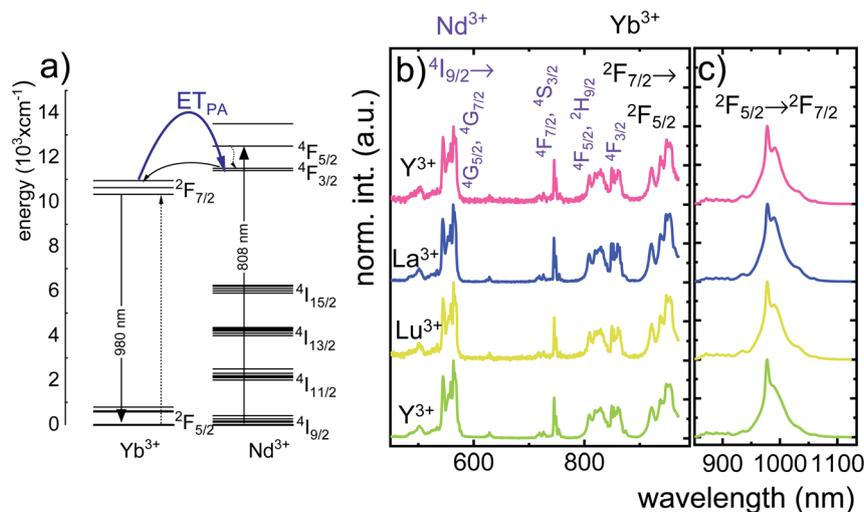
Fig. 2 The schematic simplified energy level diagram of  $\text{Yb}^{3+}$  and  $\text{Nd}^{3+}$  ions in  $\text{Nd}_{0.5}\text{RE}_{0.4}\text{Yb}_{0.1}\text{PO}_4$  (a), comparison of the normalized excitation spectra monitored at the emission of  $\text{Yb}^{3+}$  ions at  $\lambda_{\text{em}} = 980$  nm (b) and emission spectra upon  $\lambda_{\text{exc}} = 808$  nm (c) for different  $\text{Nd}_{0.5}\text{RE}_{0.4}\text{Yb}_{0.1}\text{PO}_4$  nanocrystals.
