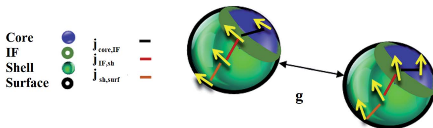
Fig. 1 Schematic representation of a system of dipolarly interacting core/shell nanoparticles. The nanoparticle architecture (soft/hard or hard/soft) defines the strength of the exchange intraparticle interactions ( j_{\text{core-IF}}, j_{\text{IF-sh}}, j_{\text{sh-surf}} ) between the four macro-spins ( S_{\text{core}}, S_{\text{IF}}, S_{\text{shell}}, S_{\text{surf}} ) for the core, shell, interface and surface regions respectively, in the mesoscopic model. Each spin also interacts with the spins of the neighbouring nanoparticles via dipolar interactions.
