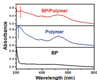
Fig. 5 UV-vis spectra of BP, polymer, and BP/polymer.
