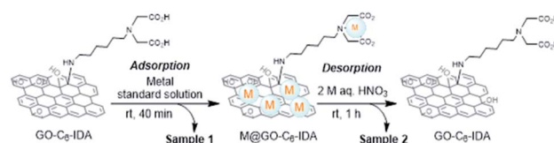
Scheme 2 Adsorption/desorption process of metal ions on/from GO–C 6 –IDA.
