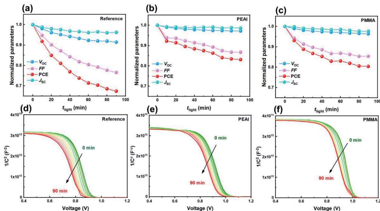
Fig. 4 Light-induced rapid degradation behavior of performance parameters of the encapsulated reference device (a), PEAI device (b) and PMMA device (c) with  $t_{\text{light}}$ , in the air at 25 °C. M–S plots of the degradation process over  $t_{\text{light}}$  of the reference device (d), PEAI device (e) and PMMA device (f) measured at 1 kHz and in the air at 25 °C.
