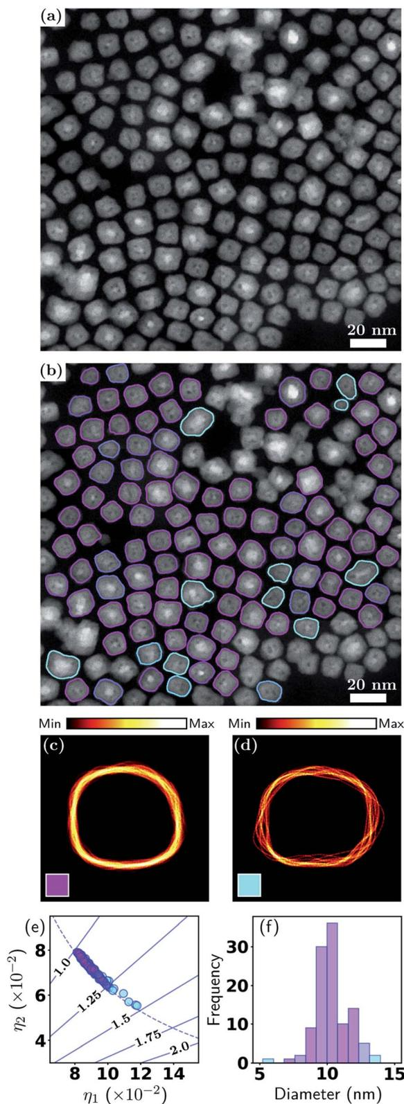
Fig. 4 Metrology of Fe–Fe<sub>2</sub>O<sub>3</sub> nanocubes. (a) ADF-STEM image and (b) with particle contours overlaid; (c and d) contour densities; (e) particle shape eigenvalues; (f) effective diameter distribution. See Section 3.1 and Fig. 2 for detailed explanations.
