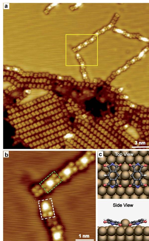
**Fig. 3** STM images of PMDI on Cu(111) after annealing to 485 K. (a) Overview STM image (0.3 V, 30 pA). (b) Zoomed-in STM image at the area marked by yellow square in (a) (0.3 V, 50 pA). A PMDI'-Cu dimer and a PMDI'-Cu monomer was highlighted by rectangle in green and in white, respectively. (c) Ball-and-stick optimized DFT model of a PMDI'-Cu dimer on Cu(111) surface, top view (top) and side view (bottom).
