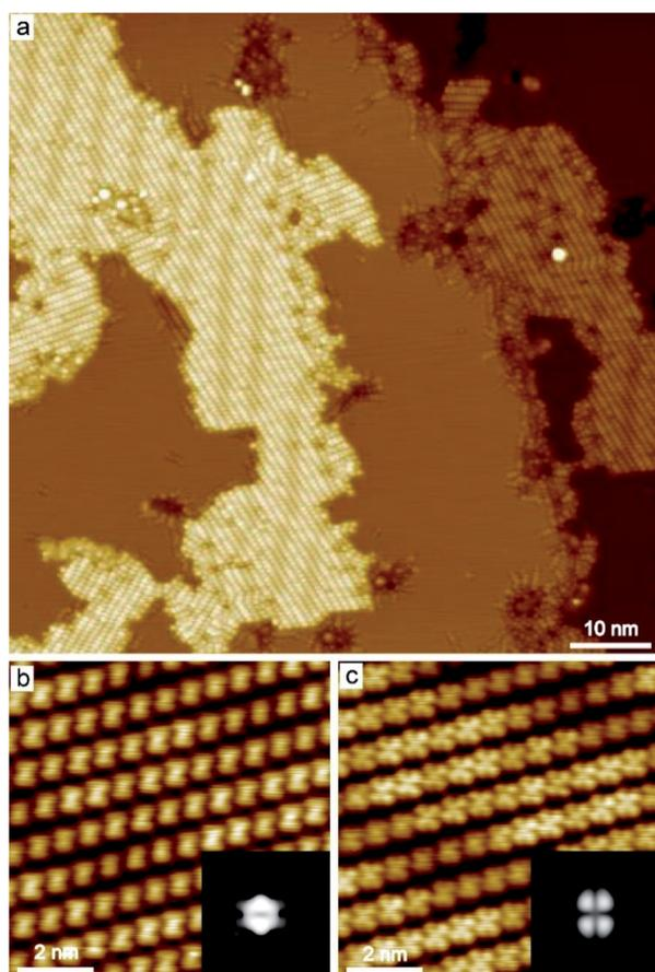
**Fig. 2** STM images of PMDI on Cu(111) surface after annealing to 405 K. (a) Overview STM image (0.5 V, 10 pA), (b) and (c) zoomed-in STM images of the same area obtained at different scanning bias ((b)  $-0.2$  V, 100 pA, the inset; (c) 1 V, 100 pA). The inset simulation STM images of PMDI' in (b) and (c) was obtained based on the optimized DFT model shown in Fig. 1d at  $-0.2$  V and 1 V, respectively.
