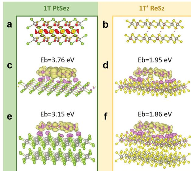
Fig. 1 The interlayer differential charge density of bilayer PtSe<sub>2</sub> (a) and bilayer ReS<sub>2</sub> (b) calculated by DFT. Side views of the electron density difference isosurface (0.00036 electron bohr<sup>-3</sup>) for MeB molecules absorbed on 1L PtSe<sub>2</sub> (c), 2L PtSe<sub>2</sub> (e), 1L ReS<sub>2</sub> (d), and 2L ReS<sub>2</sub> (f). The binding energy of these systems was calculated respectively.
