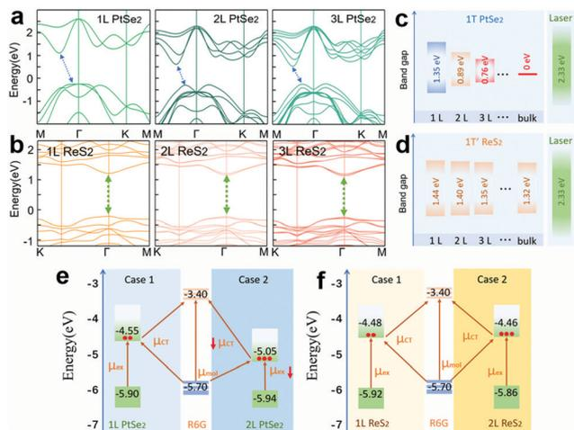
**Fig. 2** The calculated band structure of 1L, 2L, 3L PtSe<sub>2</sub> (a) and 1L, 2L, 3L ReS<sub>2</sub> (b). The energy gap at point  $\Gamma$  of PtSe<sub>2</sub> (c) and ReS<sub>2</sub> (d) from 1L to bulk. (e and f) Schematic illustration of the PICT process of the PtSe<sub>2</sub>-R6G system and ReS<sub>2</sub>-R6G system while the number of layers increased.
