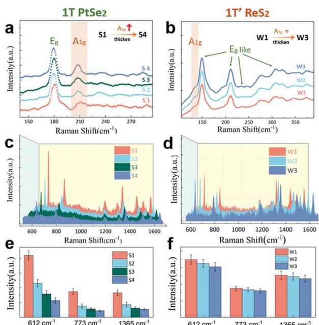
Fig. 5 Characteristic Raman spectra of (a) PtSe<sub>2</sub> films (S1 to S4) and (b) ReS<sub>2</sub> films (W1 to W3). Enhanced Raman spectra of 10<sup>-5</sup> M R6G on the (c) PtSe<sub>2</sub> films (S1 to S4) and (d) ReS<sub>2</sub> films (W1 to W3). The extracted average signal intensities integrated at 612 cm<sup>-1</sup>, 773 cm<sup>-1</sup> and 1365 cm<sup>-1</sup> for S1 to S4 (e) and W1 to W3 (f).
