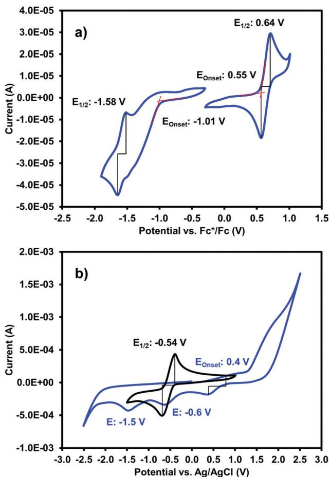
Fig. 2 (a) The cyclic voltammogram for  $(^i\text{PrNH})_2\text{NDI-V}$  measured in DCM with 0.1 M  $\text{NBu}_4\text{PF}_6$  electrolyte. Oxidation and reduction onsets and  $E_{1/2}$  potentials are shown. (b) The cyclic voltammograms for  $(^i\text{PrNH})_2\text{NDI-V}$  (blue trace) and NDI-V (black trace) measured in water with a 40% v/v 0.1 M NaCl electrolyte at pH 8.
