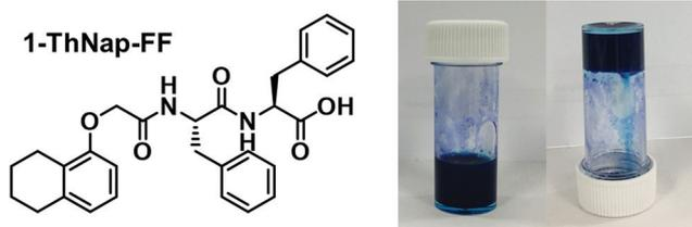
Fig. 6 The chemical structure of 1-ThNap-FF and photographs of the blend  $(^i\text{PrNH})_2\text{NDI-V}$  (5 mg mL<sup>-1</sup>) and 1-ThNap-FF (5 mg mL<sup>-1</sup>) hydrogel.
