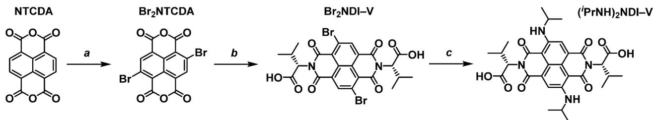
**Scheme 2** The synthetic method to obtain core-functionalised blue (iPrNH)<sub>2</sub>NDI-V. (a) Dibromoisocyanuric acid (2.5 eq.), H<sub>2</sub>SO<sub>4</sub>-20% SO<sub>3</sub>, 25 °C, 5 h, 29% yield. (b) L-Valine (2 eq.), glacial acetic acid, 120 °C, 18 h, 76% yield. (c) Isopropylamine, 25 °C, 10 days, 80% yield.
