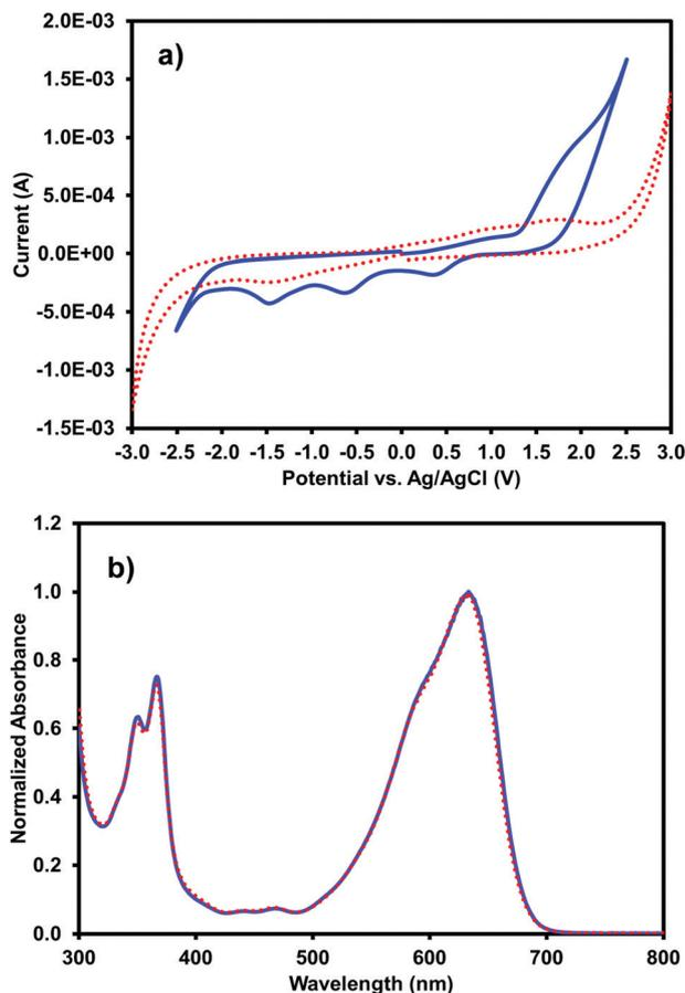
Fig. 7 (a) Cyclic voltammograms for  $(^1\text{PrNH})_2\text{NDI-V}$  measured as a solution (solid blue line) in water at pH 10 with 40% 0.1 M NaCl electrolyte and as a hydrogel (red dotted line) with 1-ThNap-FF and 40% 0.1 M NaCl electrolyte; (b) UV-vis absorption profiles for  $(^1\text{PrNH})_2\text{NDI-V}$  measured as a solution (solid blue line) in water at pH 10 and as a gel with 1-ThNap-FF (red dotted line).
