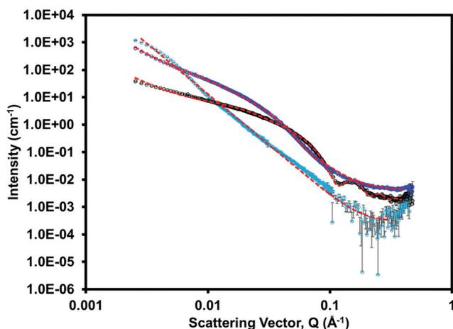
Fig. 8 Small angle neutron scattering (SANS) for the single component  $(^1\text{PrNH})_2\text{NDI-V}$  solution (light blue), single component 1-ThNap-FF gel (black), and multicomponent 1-ThNap-FF +  $(^1\text{PrNH})_2\text{NDI-V}$  gel (dark blue) with fit lines for each shown in red.
