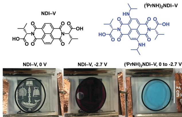
Fig. 1 The chemical structures of NDI-V and  $(^i\text{PrNH})_2\text{NDI-V}$  along with a display of the electrochromic properties of NDI-V and the lack of electrochromic properties of  $(^i\text{PrNH})_2\text{NDI-V}$ . Both species were dissolved in water with 40% v/v 0.1 M NaCl electrolyte at pH 8.
