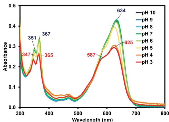
Fig. 4 The UV-vis absorption profile for  $(^1\text{PrNH})_2\text{NDI-V}$  measured in water with a 40% v/v 0.1 M NaCl at various pH values from pH 10 to pH 3 with absorption maxima shown at pH 10 (blue) and pH 3 (red).
