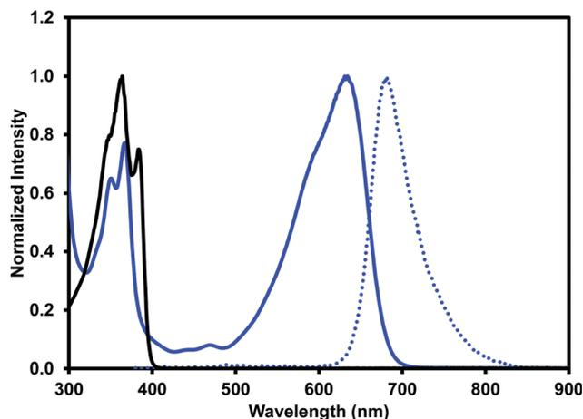
Fig. 3 The absorption (solid blue) and emission (dot blue) profiles for  $(^1\text{PrNH})_2\text{NDI-V}$  and absorption (solid black) profile for NDI-V. All spectra were measured in water with a 40% v/v 0.1 M NaCl electrolyte at pH 10. Emission profile was obtained with excitation at 360 nm.
