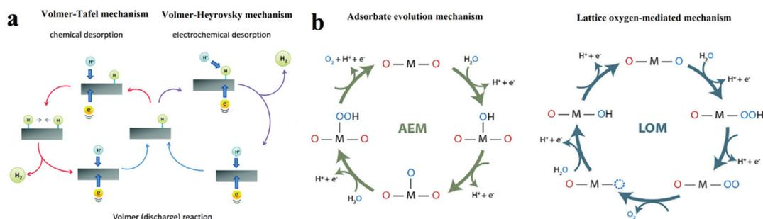
**Fig. 1** (a) The schematic of electrocatalytic turn-over of hydrogen evolution on the surface of an electrode.<sup>21</sup> (b) The adsorbate evolution mechanism (AEM) and lattice oxygen mediated mechanism (LOM) of oxygen evolution turnover on the surface of catalyst.<sup>23</sup>
