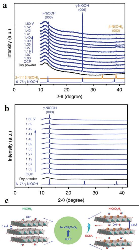
**Fig. 5** (a and b) *Operando* XRD patterns collected on (a) Ni(OH)<sub>2</sub>/NF and (b) NiCeO<sub>x</sub>H<sub>y</sub>/NF electrodes at different potentials. (c) The OER proceeds more favourably on NiCeO<sub>x</sub>H<sub>y</sub> with larger interlamellar spacing and higher ECSA relative to Ni(OH)<sub>2</sub>.<sup>59</sup>
