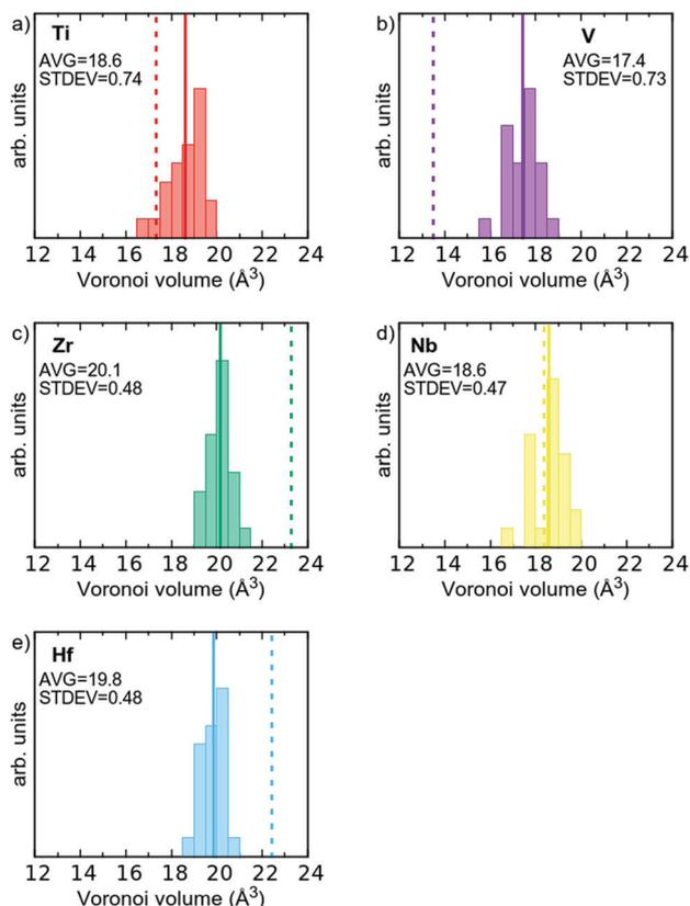
Fig. 5 Histograms of atomic volumes using the Voronoi approach in the relaxed multi-component alloy, per element type for all 120 atoms in the simulated supercell. Average volume indicated by the solid lines. Atomic volume of respective elemental reference phase given as dashed vertical lines.
