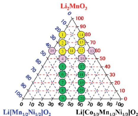
Fig. 5 Summary of the dependence of the difference in discharge capacity obtained at the 10<sup>th</sup> cycle on the targeted composition of the LLO samples. The difference in discharge capacity = (discharge capacity of the LLO sample prepared by the quenched cooling) – (discharge capacity of the LLO sample prepared by slow cooling). The difference in discharge capacities: ● > 10 mA h g<sup>-1</sup>, ● -10 mA h g<sup>-1</sup> < ● < 10 mA h g<sup>-1</sup>, ● < -10 mA h g<sup>-1</sup>.
