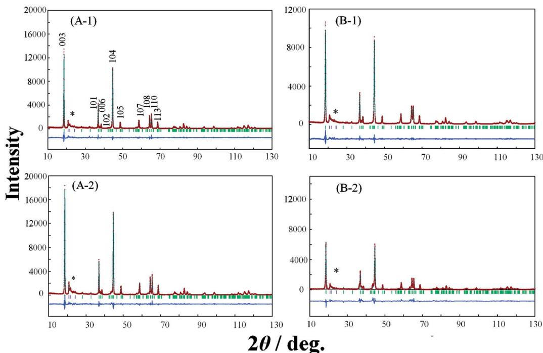
Fig. 6 XRD Rietveld refinement profiles of samples 1 (A-1, A-2) and 3 (B-1, B-2) prepared by (A-1, B-1) the quenched cooling with liquid nitrogen, and (A-2, B-2) the slow cooling in the furnace at a controlled rate of 25 °C h<sup>-1</sup>. (—) observed, (—) calculated, (—) the difference of both. The green vertical marks indicate the position of the Bragg reflections. \* corresponds to the peaks around 20–25° that result from the ordering of Li<sup>+</sup> ions in the transition metal layers.
