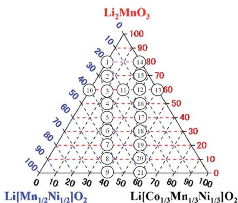
Fig. 1 Targeted compositions of synthesized LLO samples represented in the  $\text{Li}_2\text{MnO}_3$ – $\text{LiNi}_{1/2}\text{Mn}_{1/2}\text{O}_2$ – $\text{LiNi}_{1/3}\text{Mn}_{1/3}\text{Co}_{1/3}\text{O}_2$  ternary diagram. The numbers 1–21 in the circles indicate the sample number.
