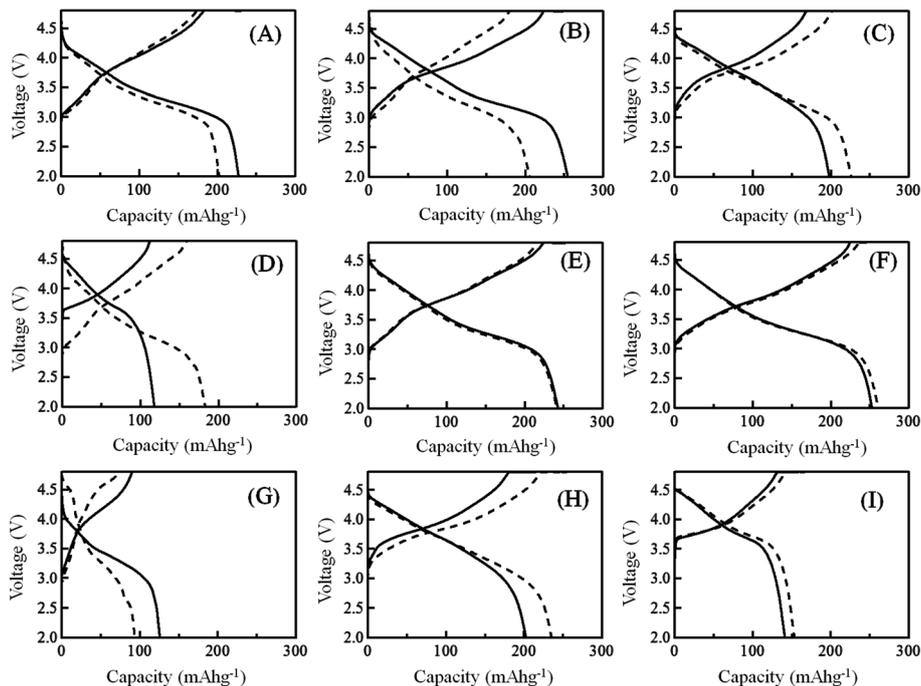
Fig. 4 Charging/discharging voltage–capacity curves obtained at the 10<sup>th</sup> cycle with samples 1 (A), 3 (B), 5 (C), 9 (D), 10 (E), 13 (F), 14 (G), 17 (H) and 21 (I) prepared by the quenched cooling with liquid nitrogen (solid lines), and the slow cooling in the furnace at a controlled rate of 25 °C h<sup>-1</sup> (dotted lines). The charging/discharging rate was 0.1C.
