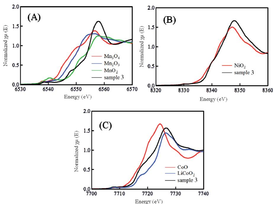
Fig. 3 (A) Mn, (B) Ni and (C) Co K-edge XANES spectra of sample 3 prepared by the quenched cooling with liquid nitrogen and reference samples of Mn<sub>3</sub>O<sub>4</sub>, Mn<sub>2</sub>O<sub>3</sub>, MnO, NiO<sub>2</sub>, CoO and LiCoO<sub>2</sub>.
