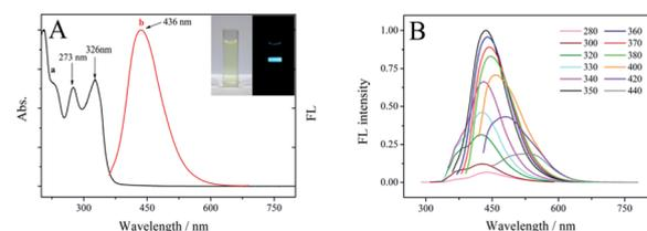
Fig. 4 (A) The normalized UV-vis absorption (a) and FL emission spectra (b) ( $\lambda_{\text{ex}} = 350$  nm) of the SUCNPs. Inset: photographs under daylight and 350 nm UV light. (B) FL emission spectra of aqueous solutions of SUCNPs with various excitation wavelengths. The slit widths were 2 nm.
