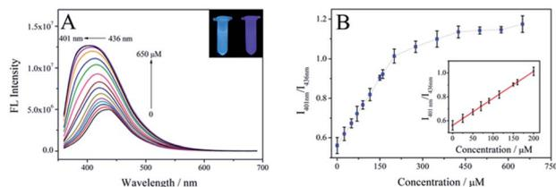
Fig. 5 (A) FL emission spectra of SUCNPs with increasing concentrations of  $\text{ClO}^-$  anions,  $\lambda_{\text{ex}} = 350$  nm, slit width = 2 nm. Inset: photographs of SUCNPs solution and SUCNP solution with the addition of  $\text{ClO}^-$  under UV light (365 nm). (B) Plots of  $I_{401 \text{ nm}}/I_{436 \text{ nm}}$  versus  $\text{ClO}^-$  concentration. Inset: the linear relationship. Error bars are shown for the standard derivation of three tests, and each RSD is lower than 5.13%.
