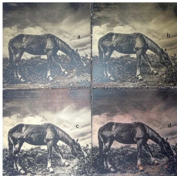
Fig. 2 Anti-corrosion effect of copperplate digital images with a superhydrophobic surface. (a) Image with a superhydrophobic surface; (b) image without a superhydrophobic surface; (c) image with a superhydrophobic film tested in an ozone aging chamber for 7 days; (d) image without a superhydrophobic film tested in an ozone aging chamber for 7 days.
