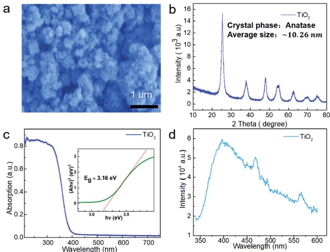
Fig. 1 (a) Scanning Electron Microscopy (SEM) image of  $\text{TiO}_2$ . (b) X-ray diffraction pattern (XRD) of  $\text{TiO}_2$ . (c) UV-visible absorption spectrum (inset: Tauc plot, shows the band gap of  $\text{TiO}_2$ :  $E_g = 3.16$  eV). (d) Photoluminescence (PL) spectrum of  $\text{TiO}_2$  at room temperature.
