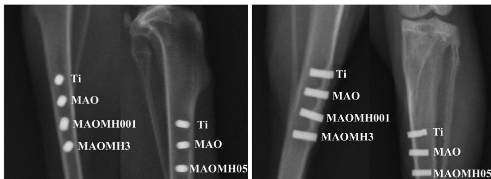
Fig. 5 X-ray images for the tibias containing the Ti, MAO, MAOMH001, MAOMH05 and MAOMH3 specimens after healing for 16 weeks.
