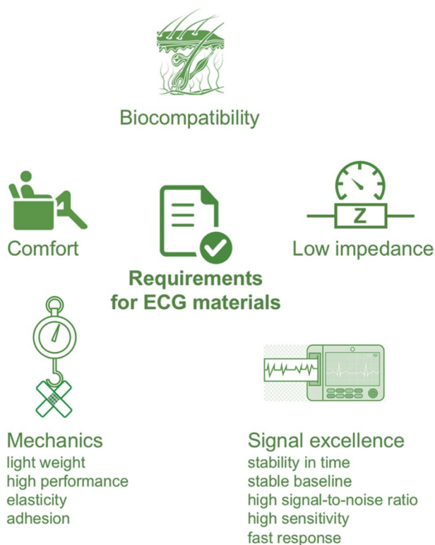
Fig. 3 The requirements for novel ECG materials.
