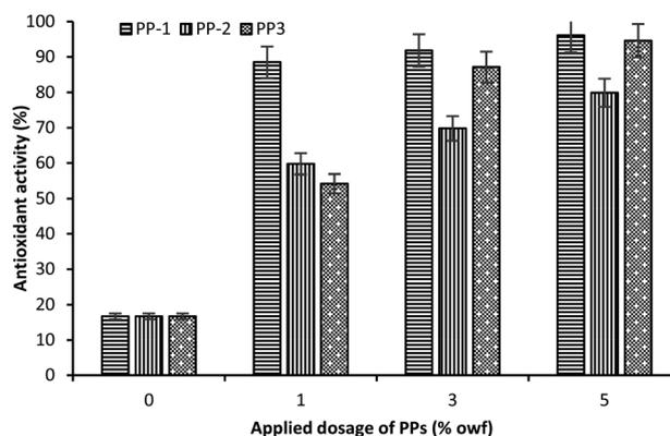
Fig. 8 Effect of applied dosage of PP on the antioxidant activity of wool fabric treated with various PPs.
