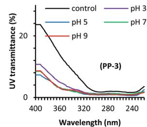
Fig. 3 Effect of treatment pH on the UV transmission of wool fabrics treated with various PPs.
