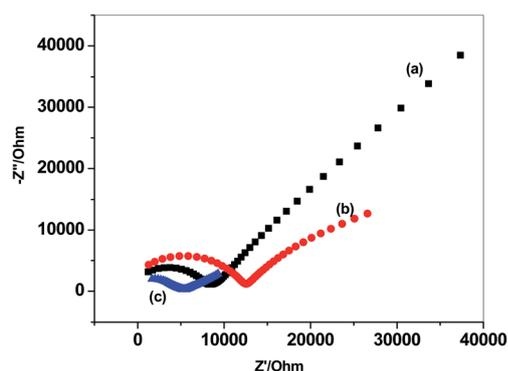
Fig. 6 Impedance plots of the C/SO<sub>3</sub><sup>2-</sup>-ISE (a), C/PANI/SO<sub>3</sub><sup>2-</sup>-ISE (b) and C/MWCNTs/SO<sub>3</sub><sup>2-</sup>-ISE (c).
