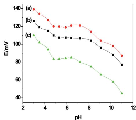
Fig. 2 pH plot for all sulfite PVC membrane-based sensors in 1 mM sulfite solution: (a) C/MWCNTs/SO<sub>3</sub><sup>2-</sup> ISE (sensor I); (b) C/PANI/SO<sub>3</sub><sup>2-</sup> ISE (sensor II); and (c) C/SO<sub>3</sub><sup>2-</sup> ISE (sensor III).
