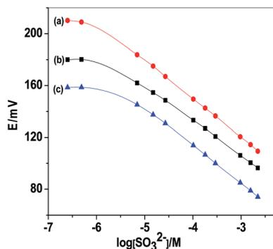
Fig. 1 Calibration plot of sulfite PVC membrane-based sensors: (a) C/MWCNTs/SO<sub>3</sub><sup>2-</sup> ISE (sensor I); (b) C/PANI/SO<sub>3</sub><sup>2-</sup> ISE (sensor II); and (c) C/SO<sub>3</sub><sup>2-</sup> ISE (sensor III).
