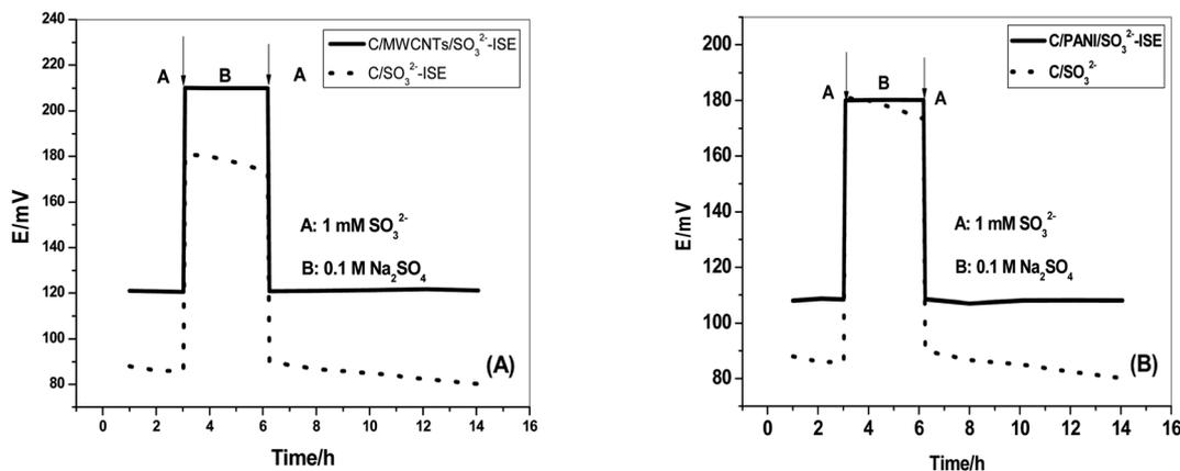
Fig. 8 Water layer tests for (A) C/MWCNTs/SO<sub>3</sub><sup>2-</sup>-ISE and (B) C/PANI/SO<sub>3</sub><sup>2-</sup>-ISE. [C/SO<sub>3</sub><sup>2-</sup>-ISE (dotted line)].
