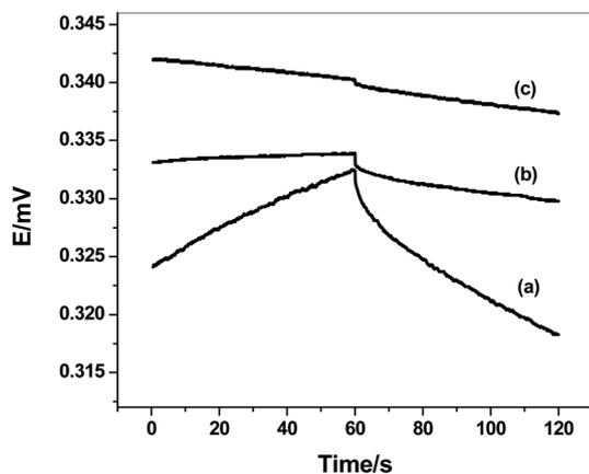
Fig. 5 Chronopotentiometry for sulfite-ISEs (a) C/SO<sub>3</sub><sup>2-</sup> ISE (sensor III); (b) C/MWCNTs/SO<sub>3</sub><sup>2-</sup> ISE (sensor I) and (c) C/PANI/SO<sub>3</sub><sup>2-</sup> ISE (sensor II).
