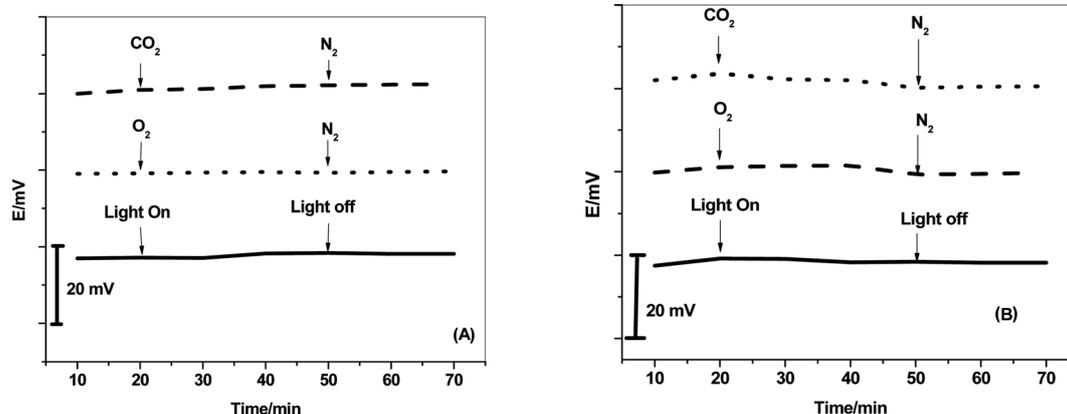
Fig. 7 Effects of CO<sub>2</sub>, O<sub>2</sub> and light on the potential stability of (A) C/MWCNTs/SO<sub>3</sub><sup>2-</sup>-ISE and (B) C/PANI/SO<sub>3</sub><sup>2-</sup>-ISE.
