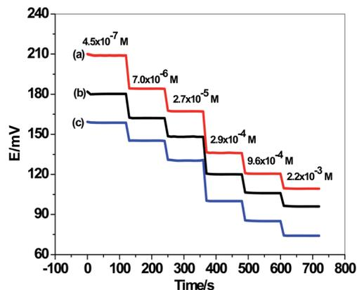
Fig. 3 Real-time potentiometric response of the developed ion-selective electrodes. (a) C/MWCNTs/SO<sub>3</sub><sup>2-</sup> ISE (sensor I); (b) C/PANI/SO<sub>3</sub><sup>2-</sup> ISE (sensor II); and (c) C/SO<sub>3</sub><sup>2-</sup> ISE (sensor III).
