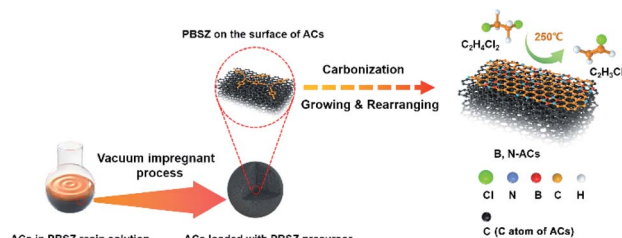
Scheme 2 Schematic representation of the synthesis of B,N-ACs.
