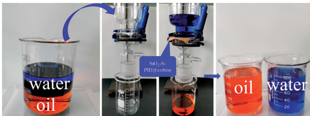
Fig. 11 Photographs of the oil–water separation process with \text{SiO}_2\text{-S-PIH@ cotton} .
