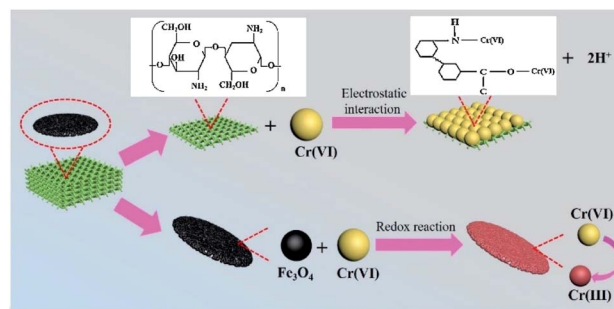
Fig. 9 Schematic illustration of the removal mechanism of Cr(VI) on Fe 3 O 4 @bagasse@chitosan (FBC) aerogel. This figure has been adapted/reproduced from ref. 89 with permission from Elsevier, under the license number 4957791186831, copyright 2020.
