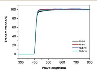
Fig. 9 UV-vis spectra of different polyfluorosilicone acrylates copolymers.
