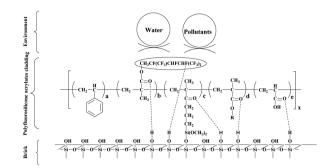
Fig. 3 Schematic diagram of the interaction between the cladding and the brick.
