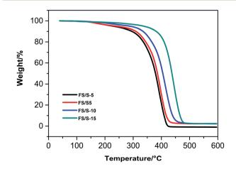
**Fig. 8** TGA curves of different polyfluorosilicone acrylates copolymers.
