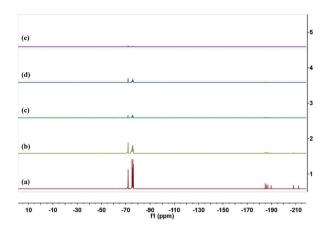
Fig. 5  $\,^{19}\mathrm{F}$  NMR spectra of (a) G04, (b) FS/S-5, (c) FS/S5, (d) FS/S-10, and (e) FS/S-15.
