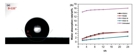
Fig. 11 (a) Water contact angle of the surface of the brick sample treated with FS/S-10; (b) the water absorption by total immersion of brick samples treated with different cladding agents.
