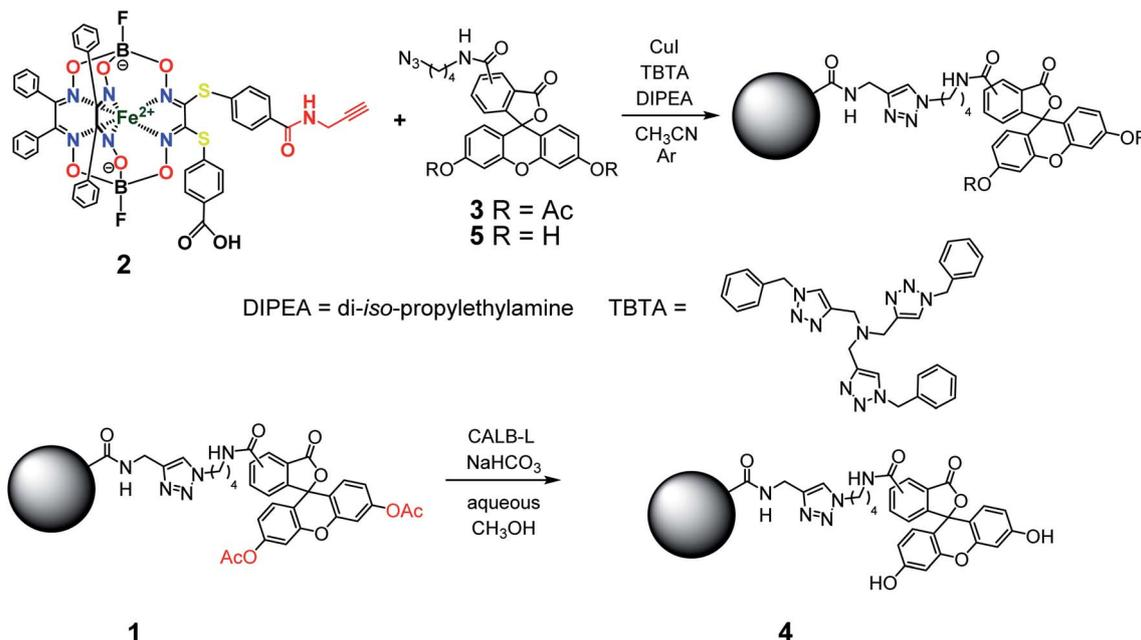
Fig. 2 Elaborated synthetic pathway to obtain a given monoribbed-functionalized iron(II) clathrochelate molecule containing a single terminal fluorescent group in one of its ribbed substituents.
