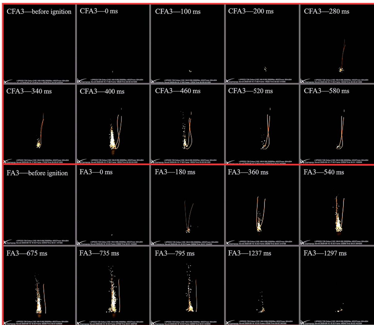
Fig. 8 High-speed photographs of Al/copper ferrites and Al/Fe 2 O 3 MICs.
