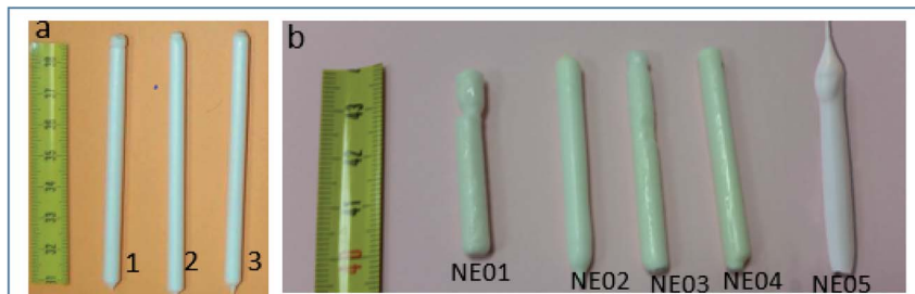
Fig. 2 \text{Al}_2\text{O}_3 -YAG- \text{ZrO}_2 ternary eutectic and off eutectic rods pulled from the melt by \mu -PD technique. (a) (1) v = 0.1 \text{ mm min}^{-1} , (2) v = 0.5 \text{ mm min}^{-1} , (3) v = 1 \text{ mm min}^{-1} . (b) (NE01 \rightarrow NE05) off eutectic rods solidified at a pulling rate of 0.5 \text{ mm min}^{-1} .
