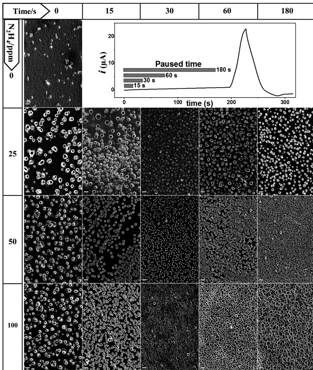
Fig. 1 SEM images of the surface of the PPy film on the ITO electrode, which was electrodeposited from different  $\text{N}_2\text{H}_4$  concentrations (rows: 0, 25, 50 and 100 ppm) and at different waiting times (columns: 0, 15, 30, 60 and 180 s) at 0.30 V. The pyrrole monomer concentration was fixed at 10 mM in the DCE solution containing 0.1 M TBAPF<sub>6</sub> as the electrolyte. Scale bar: 2  $\mu\text{m}$ .
