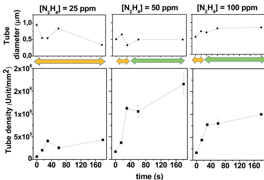
Fig. 2 Variation of the inner tube diameter and tube density at different  $N_2H_4$  concentrations as a function of the paused time at 0.30 V. The pyrrole monomer concentration was fixed at 10 mM in the DCE solution containing 0.1 M TBAPF<sub>6</sub>. The orange and green arrows indicate where the tubular structures are isolated or collapsed, respectively.
