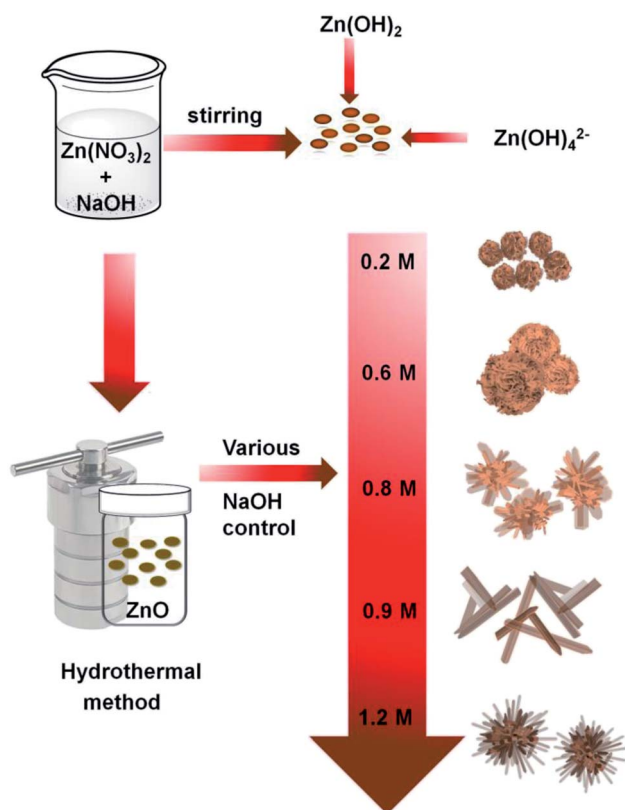
Scheme 1 Synthetic procedure for various ZnO structures.
