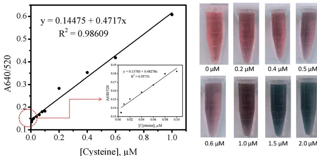
Fig. 8 The absorbance ratio of  $A_{640/520}$  (nm/nm) for the AuNPs– $\text{Cu}^{2+}$  sensing system at pH 7 over the concentration range (0.005–1.0  $\mu\text{M}$ ). The inset shows the magnified representation of  $A_{640/520}$  ratio from 0.005  $\mu\text{M}$  to 0.1  $\mu\text{M}$ . The right pictures show the progressive colorimetric changes of the AuNPs– $\text{Cu}^{2+}$  sensing system with increasing Cys concentration (0–2.0  $\mu\text{M}$ ).
