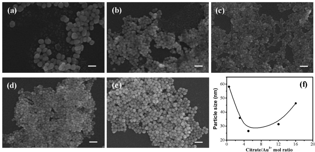
Fig. 1 SEM images of (a)–(e) AuNPs prepared using different molar ratios of citrate/Au<sup>3+</sup> (0.5, 3, 5, 12, and 16) and (f) the size variation of AuNPs with the molar ratio of citrate/Au<sup>3+</sup>. The scale bar indicates 100 nm.
