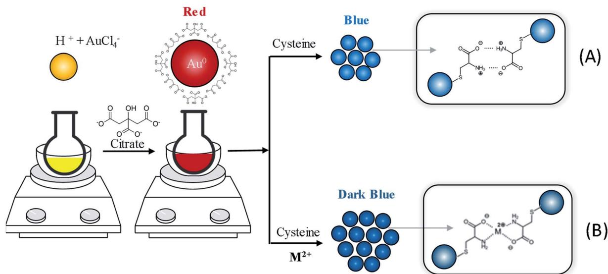
Scheme 1 Schematic illustration of aggregation behavior and color changes of AuNPs via (A) Cys-assisted cross-linking, and (B) M<sup>2+</sup>-mediated coordination complex formation.
