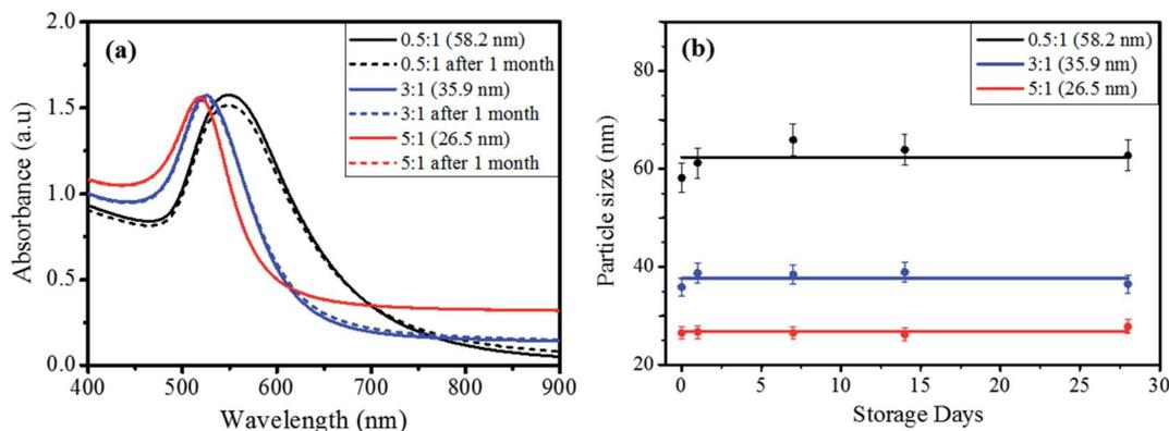
Fig. 2 (a) UV-vis spectra of AuNPs prepared with different molar ratios of citrate/Au<sup>3+</sup>, (b) the variation of particle size measured by DLS method with the elapse of storage time.
