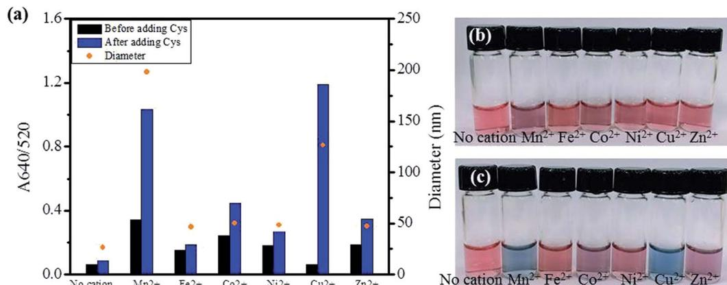
Fig. 5 The absorbance ratio of  $A_{640/520}$  in the presence of transition-metal ions at 1.0 mM before and after adding 1.5  $\mu\text{M}$  Cys at pH 7, including the particle size of aggregated AuNPs with Cys (a). The photograph of AuNPs solution before (b) and after adding Cys (c) with various cations (1.0 mM): no cation,  $\text{Mn}^{2+}$ ,  $\text{Fe}^{2+}$ ,  $\text{Co}^{2+}$ ,  $\text{Ni}^{2+}$ ,  $\text{Cu}^{2+}$ , and  $\text{Zn}^{2+}$ .
