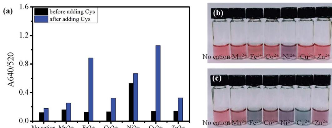
Fig. 7 The absorbance ratio of  $A_{640/520}$  in the presence of transition metal ions at 0.1 mM before and after adding 1.5  $\mu M$  Cys at pH 3.5 (a). The photograph of AuNPs solution before (b) and after adding Cys (c) with various cations (0.1 mM): no cation,  $Mn^{2+}$ ,  $Fe^{2+}$ ,  $Co^{2+}$ ,  $Ni^{2+}$ ,  $Cu^{2+}$ , and  $Zn^{2+}$ .
