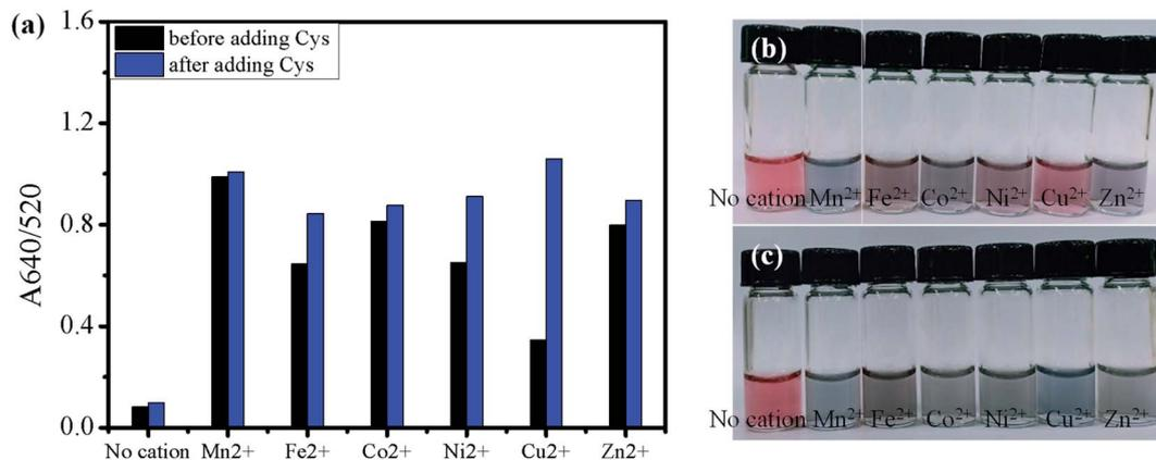
Fig. 6 The absorbance ratio of  $A_{640/520}$  in the presence of transition metal ions at 1.0 mM before and after adding 1.5  $\mu M$  Cys at pH 5 (a). The photograph of AuNPs solution before (b) and after adding Cys (c) with various cations (1.0 mM): no cation,  $Mn^{2+}$ ,  $Fe^{2+}$ ,  $Co^{2+}$ ,  $Ni^{2+}$ ,  $Cu^{2+}$ , and  $Zn^{2+}$ .
