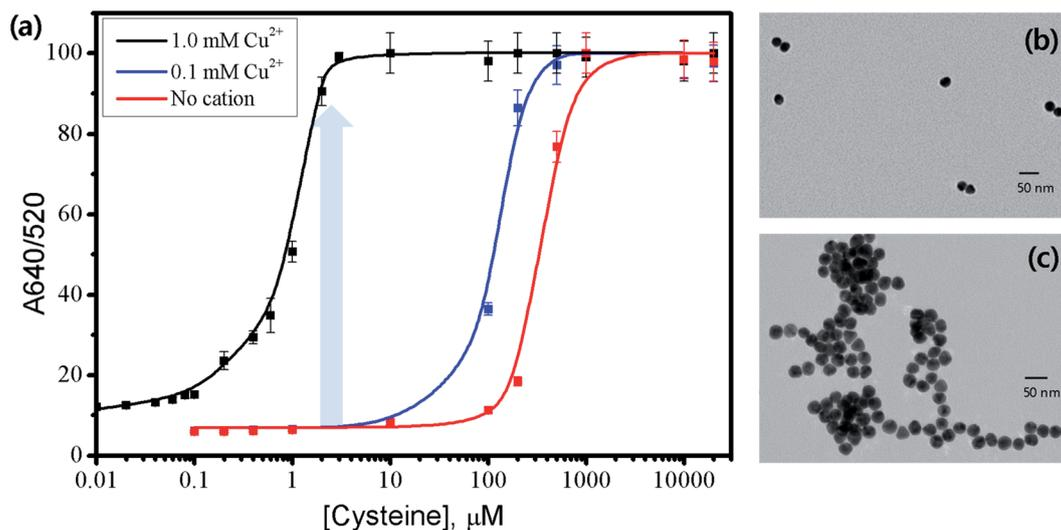
Fig. 4 (a) The absorbance ratio of  $A_{640/520}$  for the AuNPs over the concentration range of Cys between 0.005 and 20 000  $\mu\text{M}$  before and after adding  $\text{Cu}^{2+}$  ions (0.1 mM, 1.0 mM). TEM images of AuNPs with 1.5  $\mu\text{M}$  Cys (b) before and (c) after adding  $\text{Cu}^{2+}$  at 1.0 mM.
