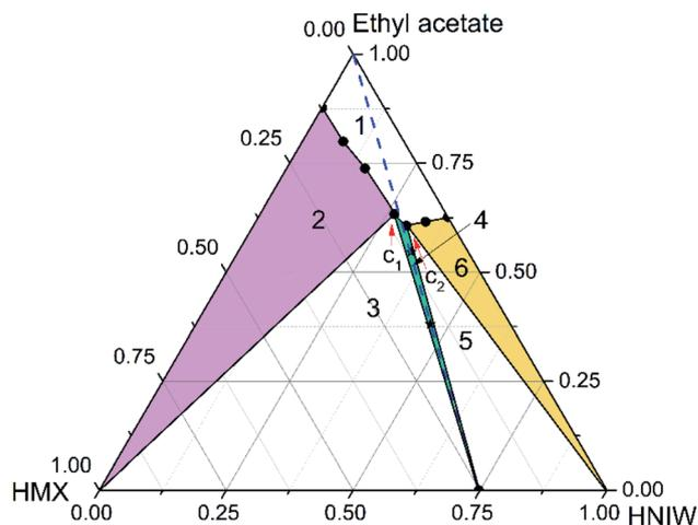
Fig. 3 Ternary phase diagram for HMX–HNIW–ethyl acetate system at 15 °C. The points (black stars) represent starting compositions for cocrystal.
