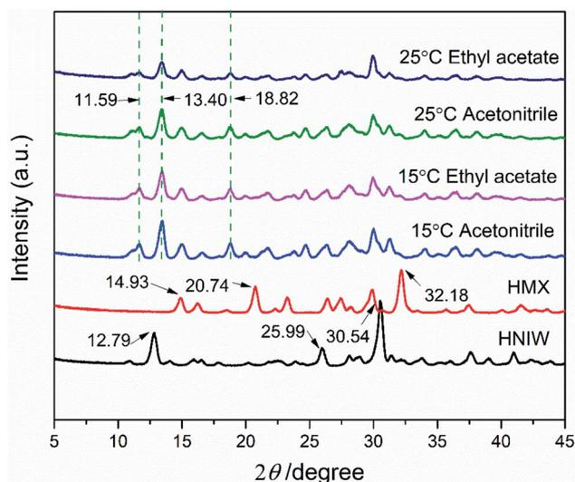
Fig. 5 PXRD patterns of 2HNIW·HMX cocrystal prepared by isothermal slurry co-crystallization method.
