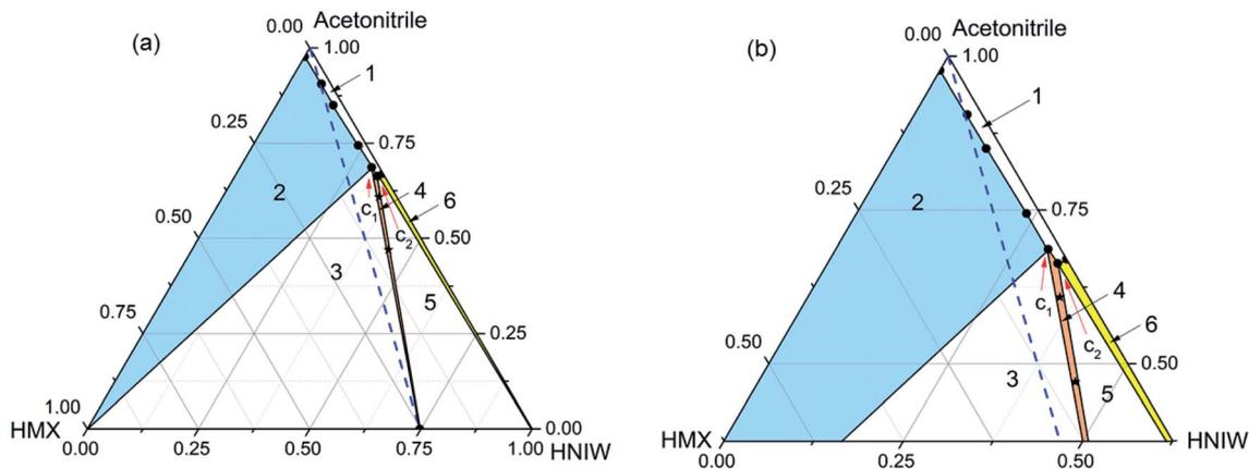
Fig. 1 Ternary phase diagram (a) and the expansion of the diagram (b) for HMX–HNIW–acetonitrile system at 15 °C. The points (black stars) represent starting compositions for cocrystal.
