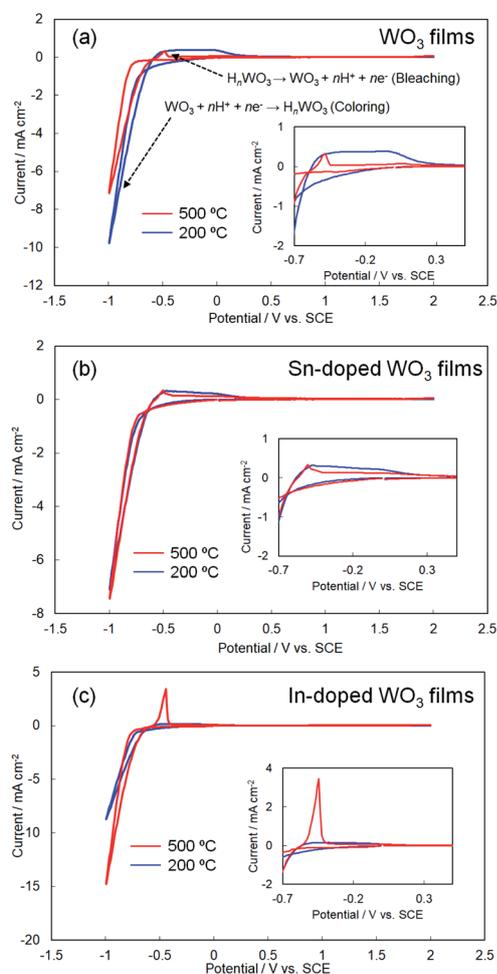
Fig. 5 Cyclic voltammograms of the  $WO_3$  (a),  $Sn-WO_3$  (b), and  $In-WO_3$  (c) films heated at  $200$  and  $500$  °C.
