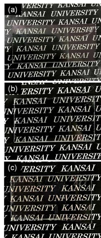
Fig. 2 Optical micrographs of the WO<sub>3</sub> (a), Sn-WO<sub>3</sub> (b), and In-WO<sub>3</sub> (c) films heated at 500 °C.
