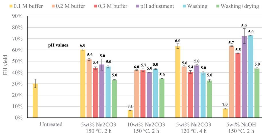
Fig. 1 Effect of various conditioning strategies on the yield from enzymatic hydrolysis of waste textiles pretreated with an alkaline solution, under 4 different conditions. Values in bold are the pH at which enzymatic hydrolysis was performed. Data represent mean values of 2 experiments; error bars indicate the spread.
