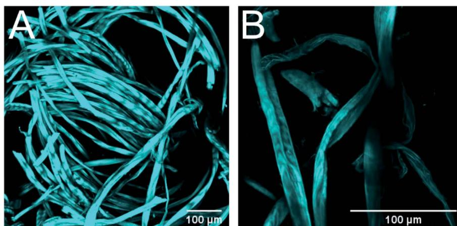
Fig. 5 CLSM images of waste textiles treated with 5%  $\text{Na}_2\text{CO}_3$  at 200 °C for 8 h. Images were taken with 20× (A) and 40× (B) magnification. Cellulose was stained with calcofluor as dye. The color was assigned arbitrarily.
