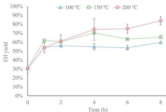
Fig. 3 Effect of the temperature and residence time on the yield from enzymatic hydrolysis of pretreated waste textiles using 5%  $\text{Na}_2\text{CO}_3$  as the alkaline solution in pretreatment. Data represent mean values of 2 experiments; error bars indicate the spread.
