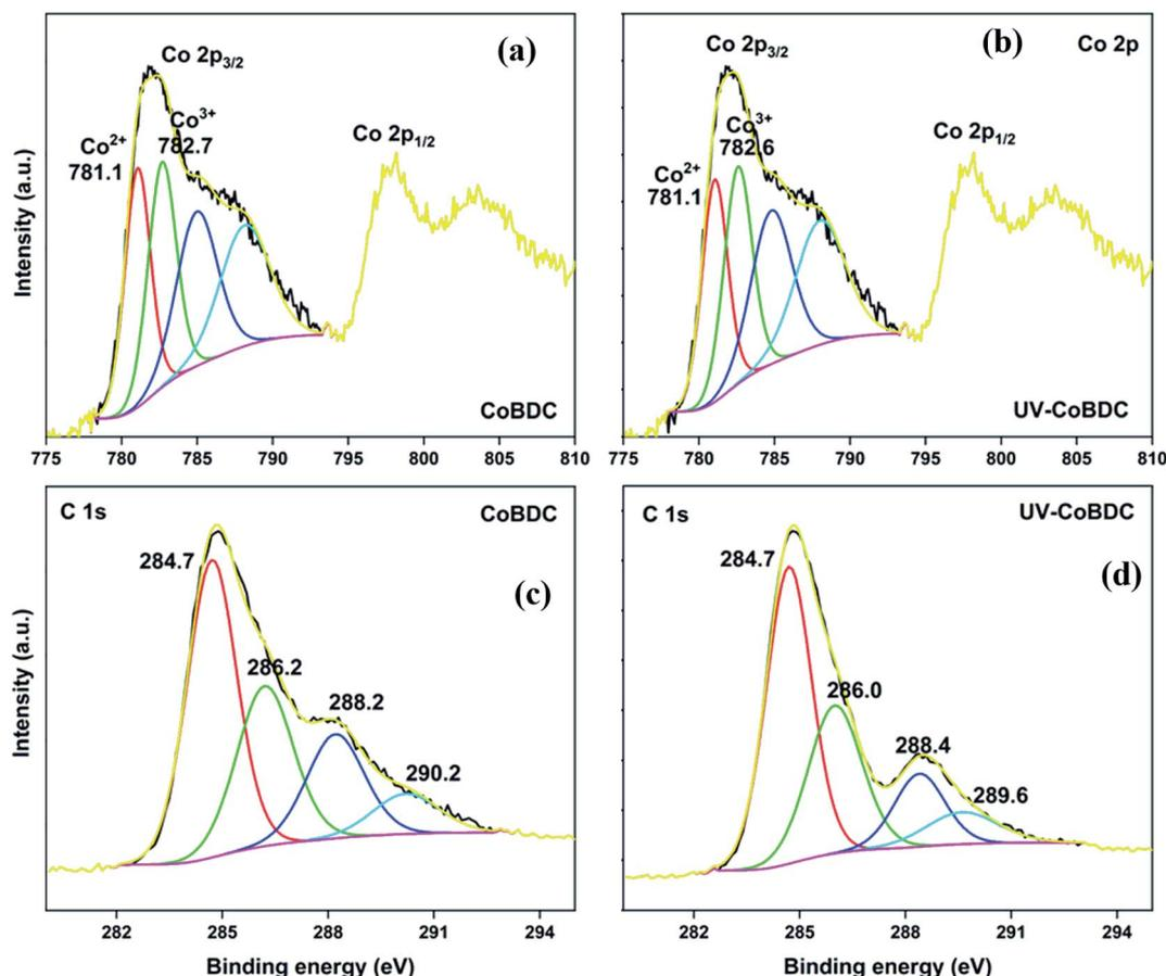
Fig. 8 HRXPS Co 2p spectra of (a) CoBDC; (b) UV-CoBDC; HRXPS C 1s spectra of (c) CoBDC; (d) UV-CoBDC.
