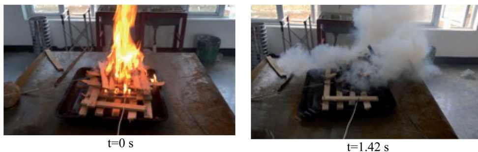
Fig. 7 Ammonium dihydrogen phosphate dry water FEA extinguishes class A fire.
