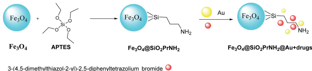
Scheme 4 The preparation of \text{Fe}_3\text{O}_4@SiO_2PrNH_2@Au + \text{drugs} .
