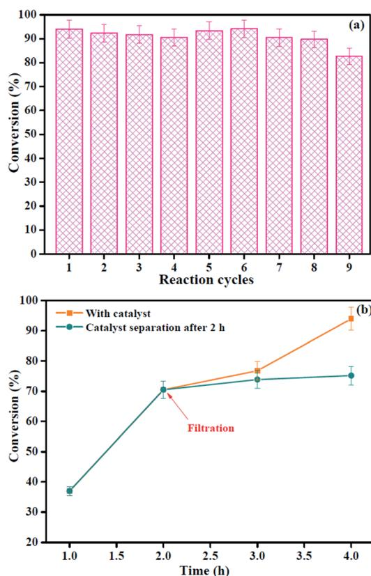
Fig. 10 (a) The OA conversion obtained by HSiW@ZrO<sub>2</sub>-300 at nine consecutive cycles of esterification reaction; (b) hot filtration test of esterification.
