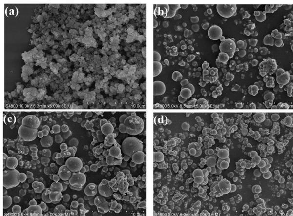
Fig. 3 SEM images for (a) HSiW@UiO-66, (b) HSiW@ZrO<sub>2</sub>-300, (c) HSiW@ZrO<sub>2</sub>-400, (d) HSiW@ZrO<sub>2</sub>-500.
