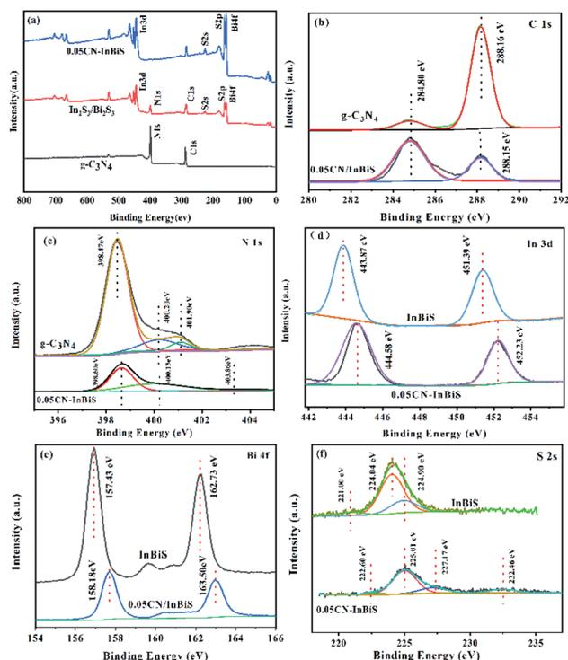
Fig. 4 XPS spectra of the CN,  $\text{In}_2\text{S}_3/\text{Bi}_2\text{S}_3$ , and  $0.05\text{CN}/\text{In}_2\text{S}_3/\text{Bi}_2\text{S}_3$ ; (a) survey, (b) C 1s, (c) N 1s, (d) In 3d, (e) Bi 4f, and (f) S 2s spectra.
