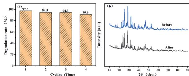
Fig. 9 (a) Cycling runs of 0.05CN/Bi<sub>2</sub>S<sub>3</sub>/In<sub>2</sub>S<sub>3</sub> in the degradation of RhB under visible light. (b) PXRD pattern of 0.05CN/Bi<sub>2</sub>S<sub>3</sub>/In<sub>2</sub>S<sub>3</sub> before and after carrying out the photocatalytic experiments.
