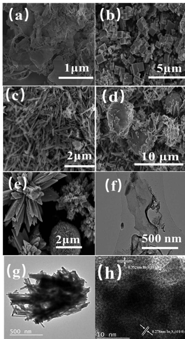
Fig. 2 SEM images of (a)  $g\text{-C}_3\text{N}_4$ ; (b)  $\text{In}_2\text{S}_3$ ; (c)  $\text{Bi}_2\text{S}_3$ ; (d)  $\text{Bi}_2\text{S}_3/\text{In}_2\text{S}_3$ ; (e)  $0.05\text{CN}/\text{Bi}_2\text{S}_3/\text{In}_2\text{S}_3$ ; TEM images of (f)  $g\text{-C}_3\text{N}_4$ ; (g)  $\text{Bi}_2\text{S}_3/\text{In}_2\text{S}_3$  and HRTEM images of (h)  $0.05\text{CN}/\text{Bi}_2\text{S}_3/\text{In}_2\text{S}_3$ .
