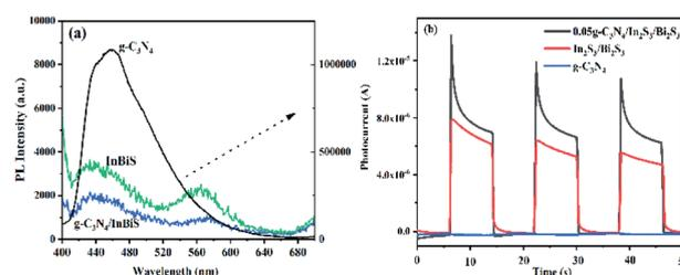
Fig. 6 PL spectra (a) and photocurrent (b) of the g-C<sub>3</sub>N<sub>4</sub>, Bi<sub>2</sub>S<sub>3</sub>/In<sub>2</sub>S<sub>3</sub> and 0.05 g-C<sub>3</sub>N<sub>4</sub>/Bi<sub>2</sub>S<sub>3</sub>/In<sub>2</sub>S<sub>3</sub> composites.
