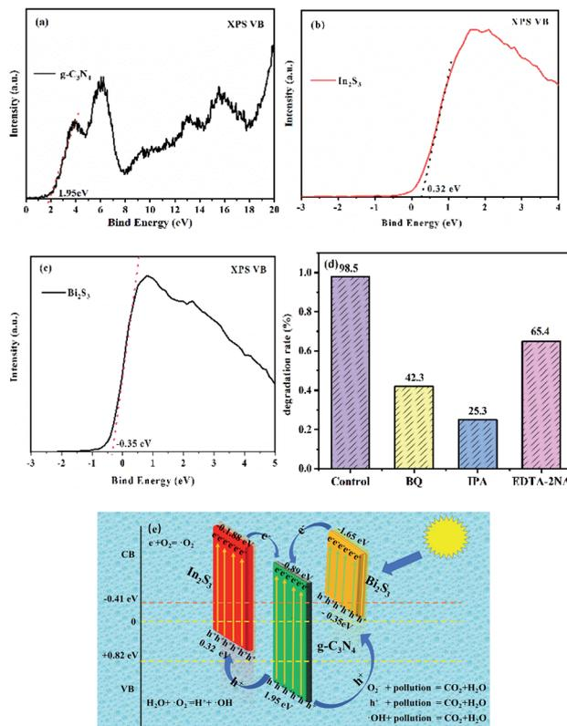
Fig. 8 (a)–(c) show the valence band diagrams of g-C<sub>3</sub>N<sub>4</sub>, In<sub>2</sub>S<sub>3</sub> and Bi<sub>2</sub>S<sub>3</sub>; (d) the free radical trapping experiments for the degradation of RhB over the 0.05CN/Bi<sub>2</sub>S<sub>3</sub>/In<sub>2</sub>S<sub>3</sub> composite. (e) The proposed photocatalytic mechanism for the degradation of RhB on the surface of the 0.05CN/Bi<sub>2</sub>S<sub>3</sub>/In<sub>2</sub>S<sub>3</sub> composite.
