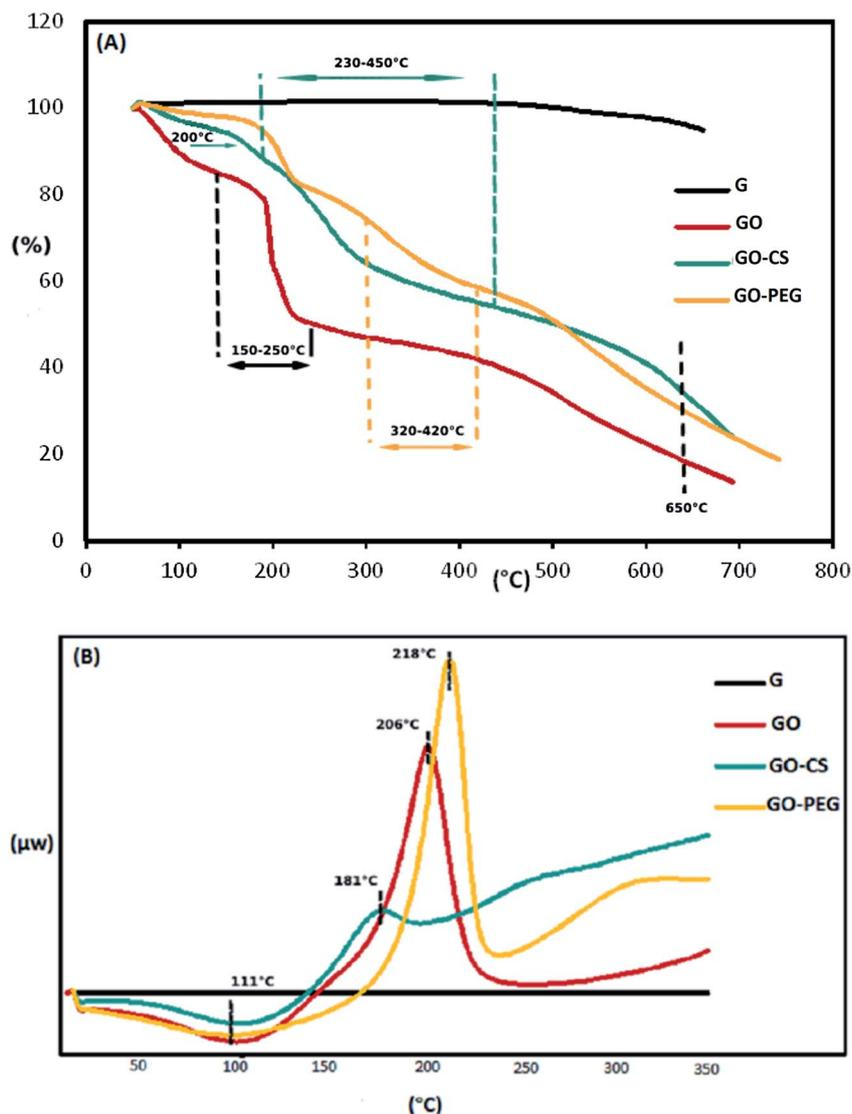
Fig. 4 TGA (A) and DSC (B) diagrams of G, GO, GO-CS and GO-PEG.
