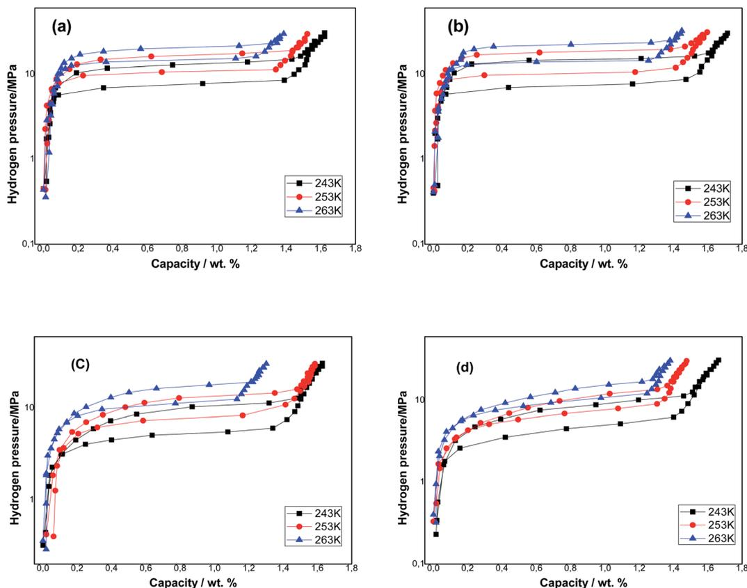
Fig. 2  $P$ - $C$ - $T$  curves of  $\text{Ti}_{1.02}\text{Cr}_{1.1}\text{Mn}_{0.3}\text{Fe}_{0.6}\text{RE}_{0.03}$  alloys: (a)  $\text{Ti}_{1.02}\text{Cr}_{1.1}\text{Mn}_{0.3}\text{Fe}_{0.6}$  alloy; (b)  $\text{Ti}_{1.02}\text{Cr}_{1.1}\text{Mn}_{0.3}\text{Fe}_{0.6}\text{La}_{0.03}$  alloy; (c)  $\text{Ti}_{1.02}\text{Cr}_{1.1}\text{Mn}_{0.3}\text{Fe}_{0.6}\text{Ce}_{0.03}$  alloy; (d)  $\text{Ti}_{1.02}\text{Cr}_{1.1}\text{Mn}_{0.3}\text{Fe}_{0.6}\text{Ho}_{0.03}$  alloy.
