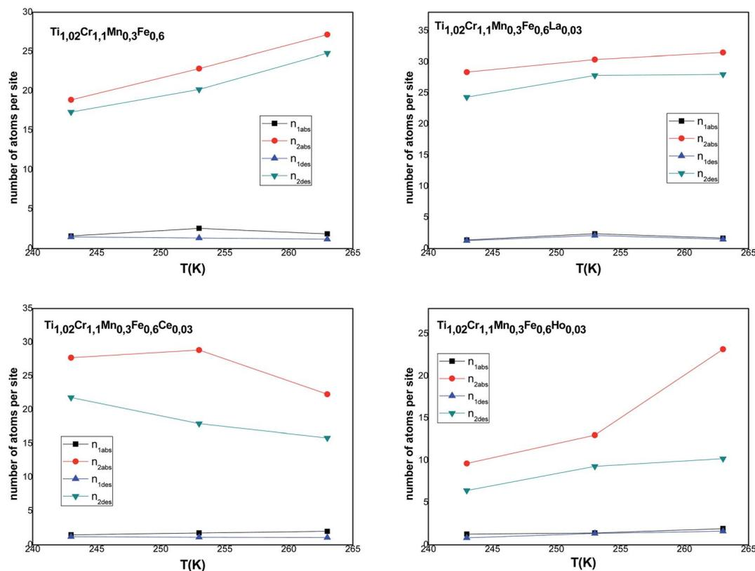
Fig. 4 Evolution of the number of atoms per site in absorption and desorption according to the temperature.
