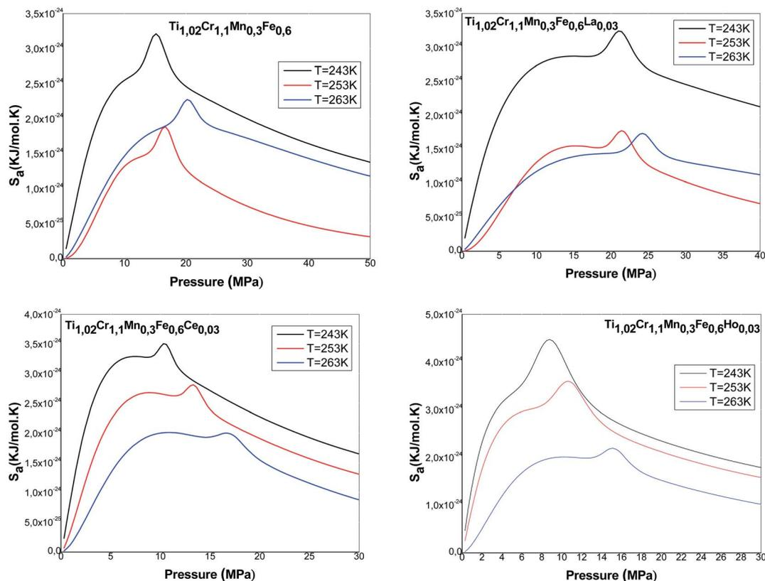
Fig. 9 Evolution of absorption entropy versus pressure.
