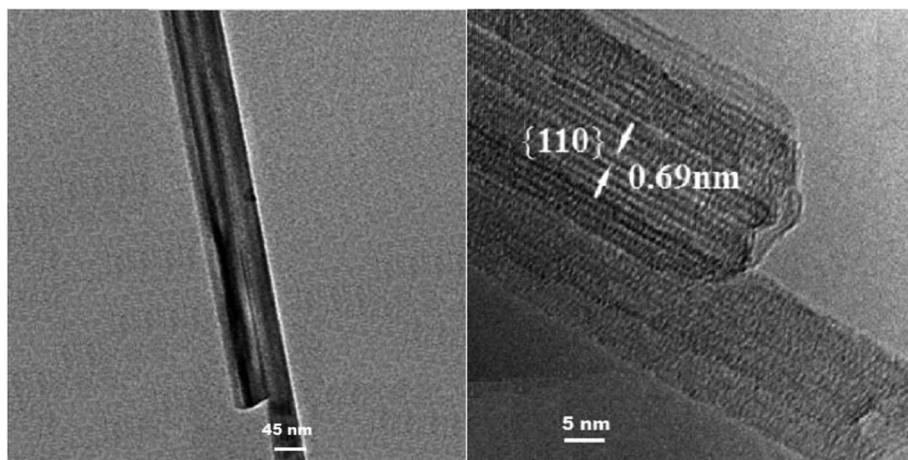
Fig. 2 High-resolution transmission electron microscope (HRTEM) images of OMS-2-SO<sub>3</sub>H.
