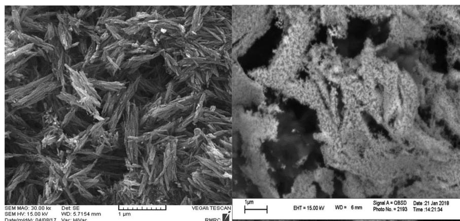
Fig. 1 SEM micrograph images of the synthesized OMS-2 (left) and sulfonated OMS-2 (right).
