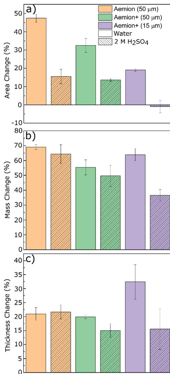
Fig. 1 Swelling behaviour of Aemion and Aemion+ membranes with sulfate counter-ions in water and 2 M  $\text{H}_2\text{SO}_4$ . (a) Area change, (b) mass change and (c) thickness change are shown with clear bar charts representing samples immersed in water and shaded bar charts representing those immersed in 2 M  $\text{H}_2\text{SO}_4$ . Wet values were taken from samples that were immersed in the appropriate liquid for 24 hours at room temperature (24  $^{\circ}\text{C}$ ).
