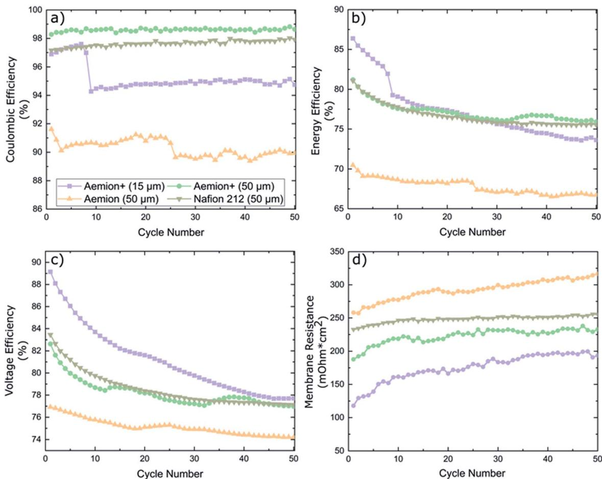
Fig. 5 Cycling data for Aemion (50 μm), Aemion+ (50 μm), Aemion+ (15 μm) and Nafion 212 (50 μm) was obtained by cycling at 100 mA cm<sup>-2</sup> with an electrode active area of 5 cm<sup>2</sup>. (a) Coulombic efficiency, (b) energy efficiency, (c) voltage efficiency and (d) membrane Ohmic resistance are reported.
