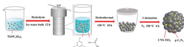
Scheme 1 Schematic illustration of the formation of the CNS-TiO 2 /g-C 3 N 4 heterojunction.
