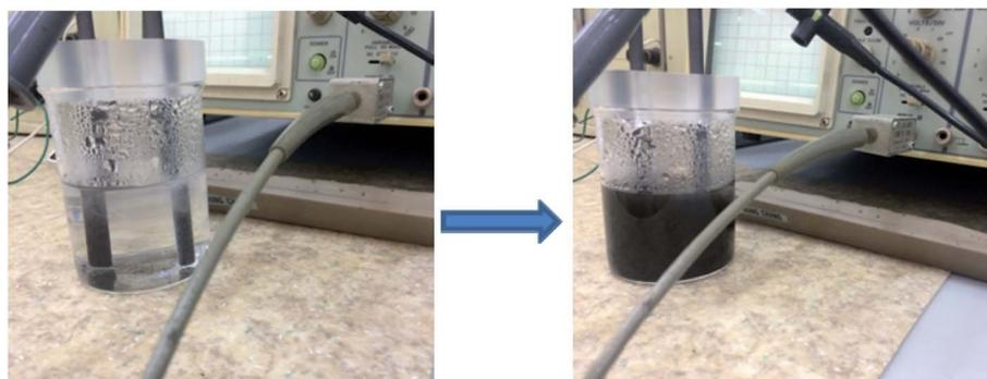
Fig. 1 Electrochemical exfoliation of graphite rods immersed in a solution containing 0.1 mol  $\text{L}^{-1}$   $\text{NH}_4\text{SCN}$  and 0.2 mol  $\text{L}^{-1}$  ammonia (applied bias 12 V; pulse duration 0.8 s; the pause between two pulses 0.2 s).
