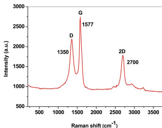
Fig. 8 The Raman spectrum of the E-NSGr sample.
