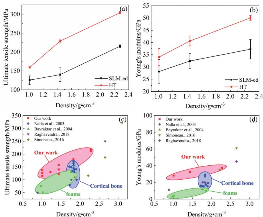
Fig. 9 (a) Tensile strength and (b) Young's modulus of the SLM-ed and HT-ed *versus* the density; (c) tensile strength and (d) Young's modulus *versus* density for various lattice structure, including our work, cortical bone, and bending-dominated lattice material.<sup>33–36</sup>
