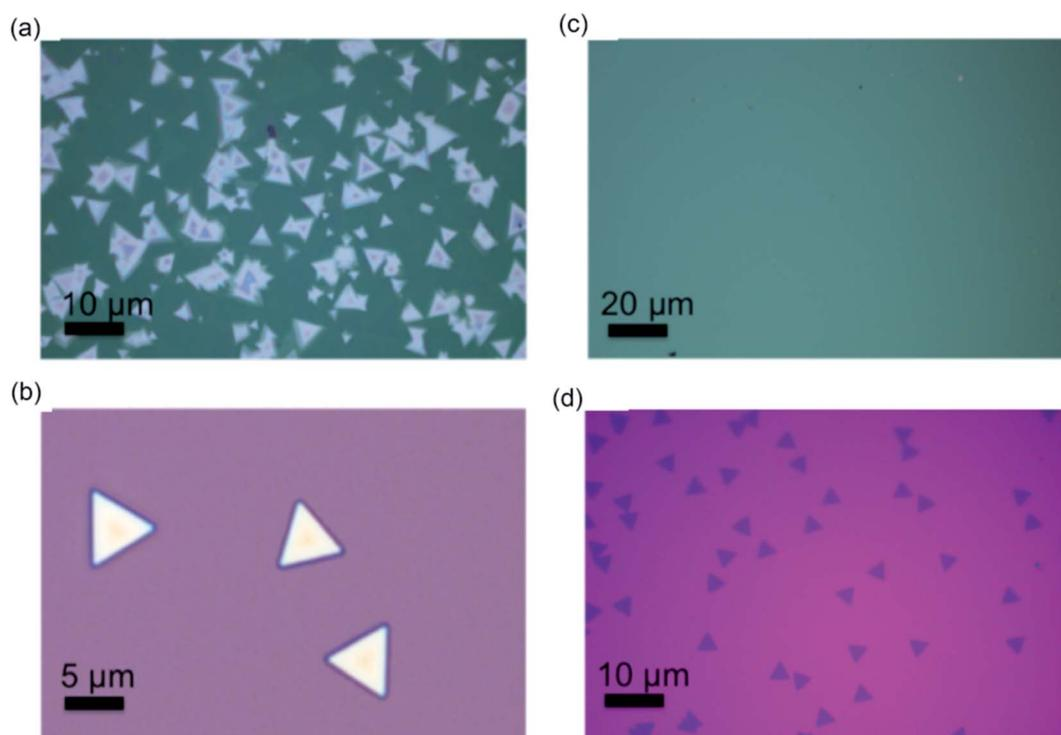
**Fig. 2** (a and b) Show the optical microscopy (OM) images of the multilayered  $\text{WSe}_2$  on the hBN film and the  $\text{SiO}_2$  substrate, respectively, at the same growth condition. (c and d) Shows the OM images of the monolayer  $\text{WSe}_2/\text{hBN}$  and  $\text{WSe}_2/\text{SiO}_2$ , respectively.
